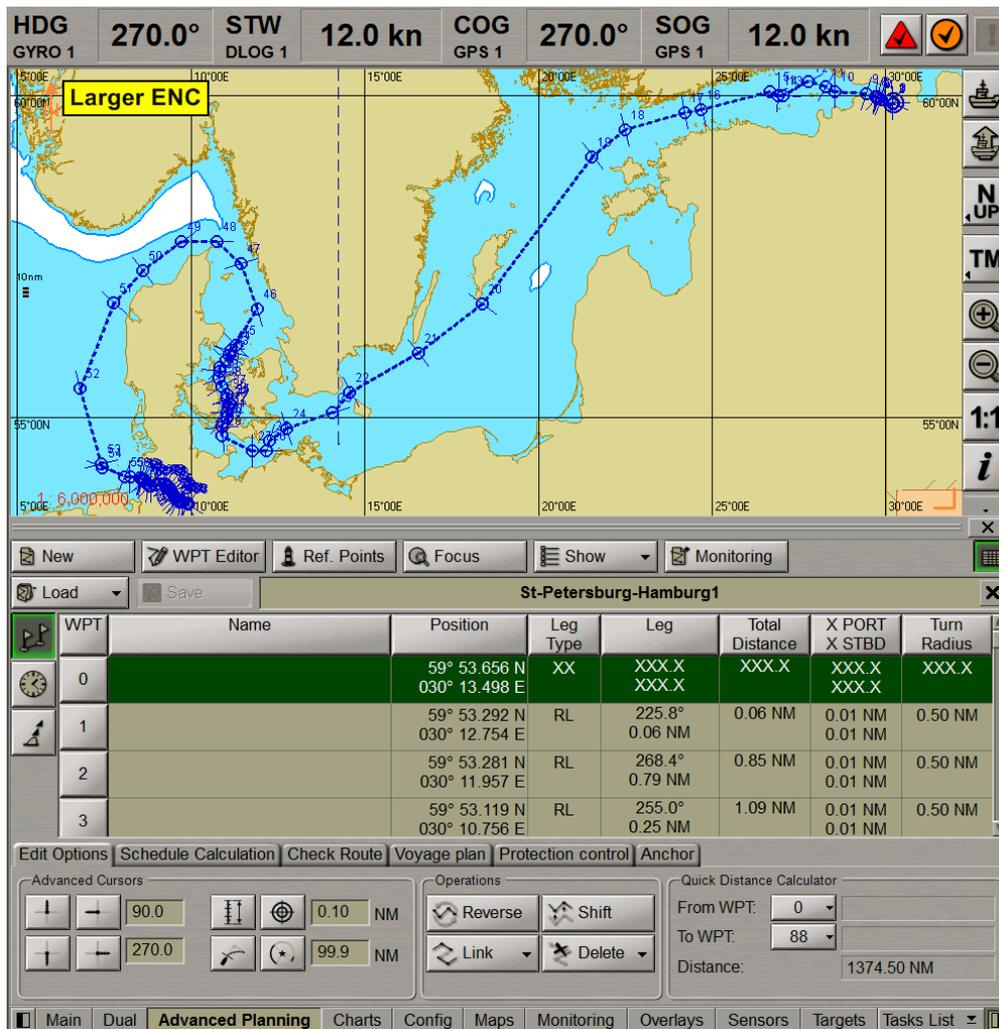
The route is displayed by superimposing a transparent layer containing route elements only, on the ECDIS task screen chart information. The following route elements are displayed on the ECDIS task Chart panel:
