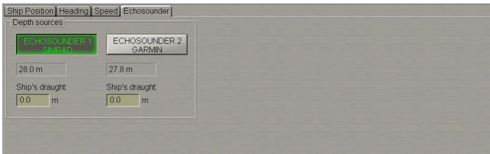
The **Echosounder** page shows all the connected depth sensors and data from the electronic chart and tidal height.
