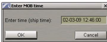
After the time has been specified, the MOB point is set in the own ship track point closest to the entered time.
