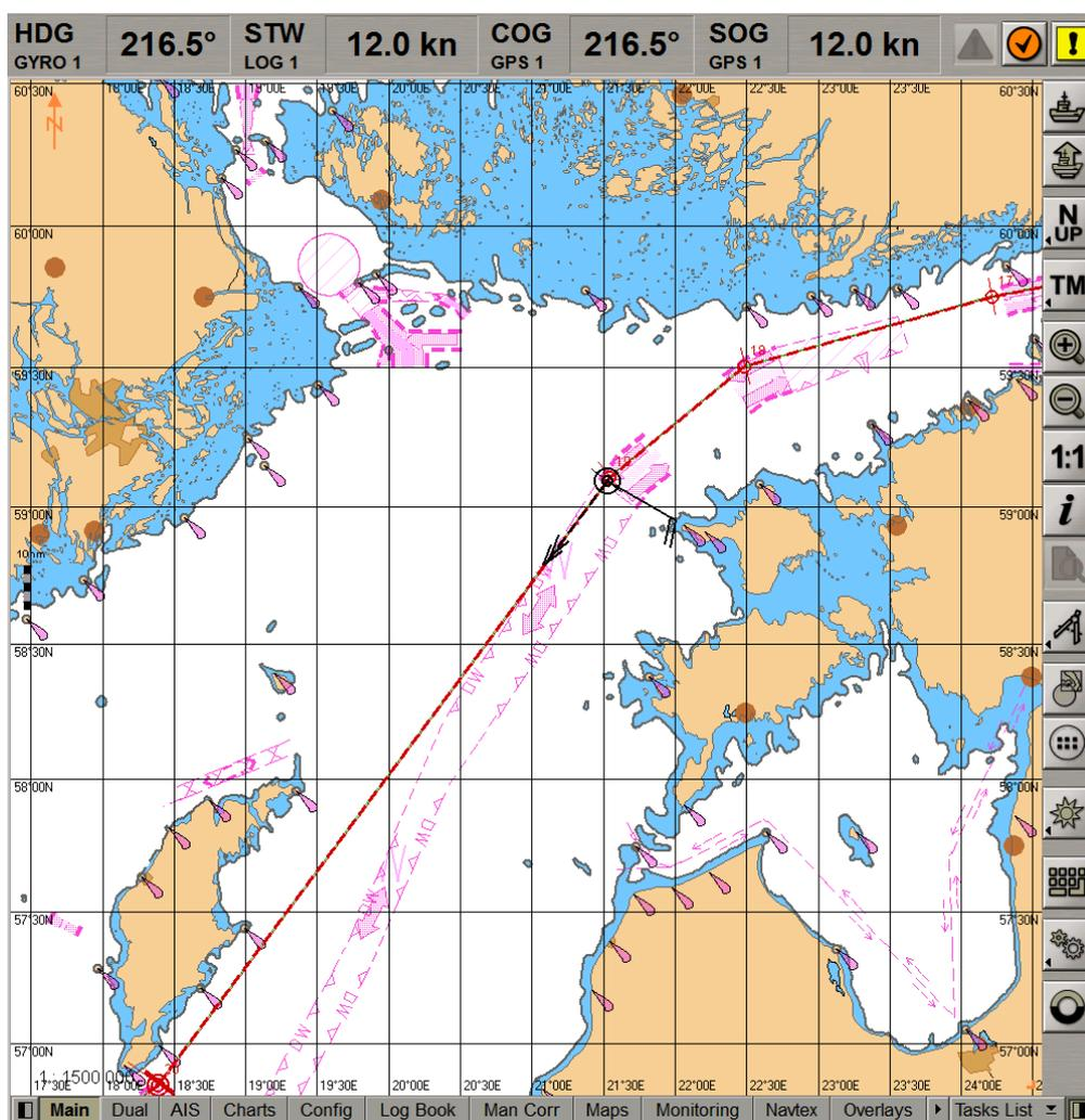
The **Main** panel is always displayed on the ECDIS task screen; the **Dual** panel is displayed by using the tab in the bottom part of the ECDIS task screen. The **Dual** panel is an additional Chart panel and serves for the navigation mode only.
