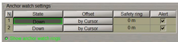
The centre of the anchor watch ring is set automatically at the moment of pressing the **Down** button, and corresponds to the anchor point position at this time. With the use of the **By Cursor** button, the user him/herself sets the anchor watch ring centre with the cursor on the Chart panel.
