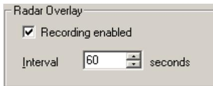
It is necessary to note that the recorded information takes up much space (memory) on the computer hard disk, which may become overfilled if a large recording duration is set.
