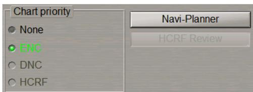
With the selected **None** checkbox, the standard ECDIS task operating mode is set, whereby all the charts from the collection in any format are equally suitable for use. In this case, if there are several charts on the same scale, priority is given to the TX-97 (TRX) format charts.
