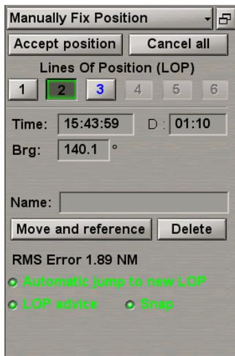
If it is necessary to accept the results of a manually fixed position, use the **Accept position** button. At the moment when the position is accepted, a "Position Fix" event is recorded, and an entry is made in the Electronic system logbook.
