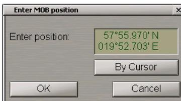
After the input of coordinates (manually or by cursor), the MOB display is re-drawn to suit the entered data (e.g., upon receipt of coordinates from another ship).
