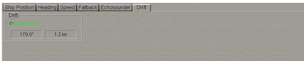
When it is disconnected (the checkbox is cleared), calculated data is used.
