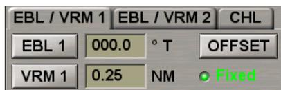
Control of the function is from the **EBL/VRM/CHL** window on the Control Panel, or from the ES6 keyboard.
