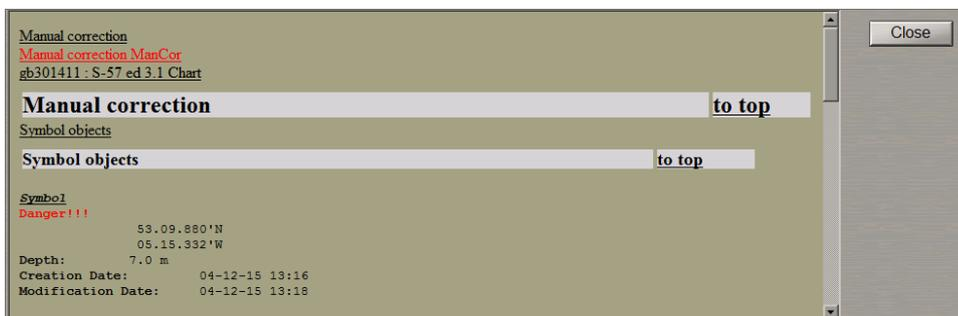
With the use of S-57 format charts, point type objects are marked with a circle if the **Highlight** function is selected on the **Info** panel. To cancel the marking, press the **Unmark** button.
