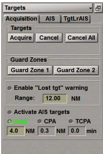
The following functions are used for handling ARPA targets on the given WS:
