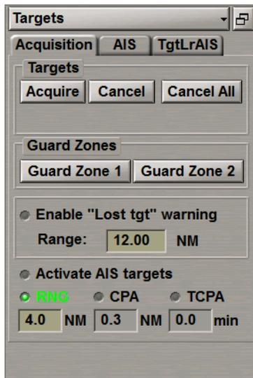
By default, the filter for activation of sleeping AIS targets is OFF. It is possible to select criteria for sleeping AIS targets activation:
