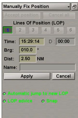
The entered data is not accepted for processing by the MFD until the **Apply** button is pressed. With the **Automatic jump to new LOP** checkbox selected, there is an automatic switch to the input of the next measurement results. In this case, the **D** box shows the time difference between the input of the first and current measurements, and it is the time which is taken into account in the ship position calculations from the position lines.
