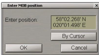
In the input box, enter the MOB coordinates: the MOB display is re-drawn to suit the entered data (e.g., upon receipt of coordinates from another ship).
