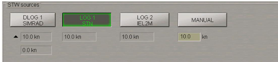
The **STW sources** group is designed for selecting a source of speed through the water. The group shows all the connected speed-through-water sensors.
