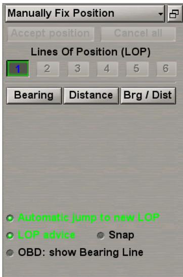
The OBD continuously transmits bearing information to the MFD. This allows the ECDIS task screen to provide a real-time display of an Optical Bearing Line – showing what the OBD operator is looking/pointing at.
