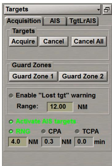
Select the **Activate AIS targets** checkbox for the automatic activation of sleeping AIS targets by one of the following criteria:
