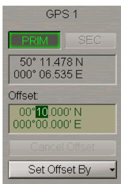
The ship symbol will move to the corrected coordinates, the coordinate offset will be displayed in the **Offset** window, whilst the position window will show corrected coordinates from the position source.
