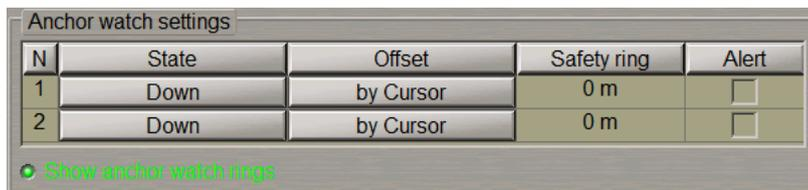
In the **Safety ring** column enter the maximum distance ( Safety ring radius) from anchor points 1 and 2. Position of anchor points 1 and 2 is set on the ship contour during the installation in the System Configuration utility. (see document *Multifunctional Display. (v. 3.02.350). Installation Guide, Chapter 2, section MFD Configuration , paragraph MFD Settings )*
