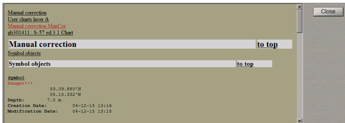
Select the **Manual correction** by positioning the cursor on this notation and press the left trackball button. The **Info** panel will display a page with information on the categories of updating objects which fall within the acquisition marker outline.
