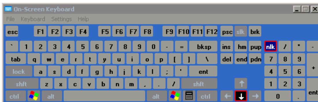
The virtual keyboard is shown in the bottom part of the Control panel and can be moved within it. To do this, position the free cursor on the virtual keyboard as shown below, and press the left trackball button. Holding the left trackball button, move the virtual keyboard to the necessary place so that it does not obscure the necessary input box.
