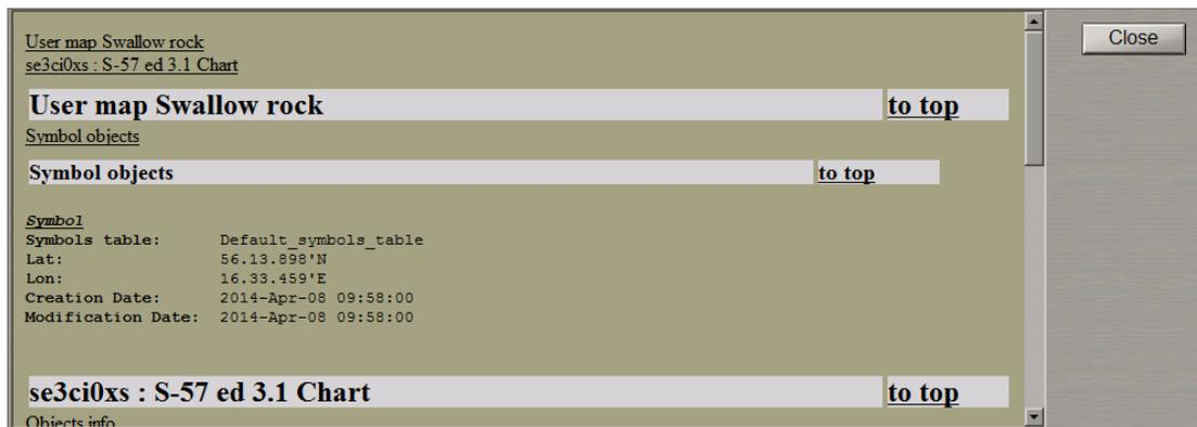
Select **User charts layer A (B)** by positioning the cursor on this notation and press the left trackball button. The **Info** panel will display a page with information on the categories of map objects which fall within the acquisition marker outline.
