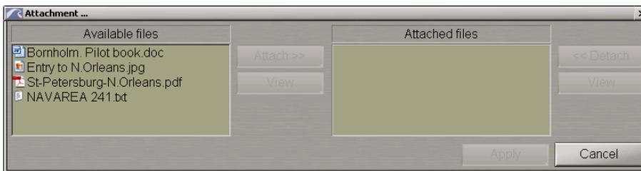
To attach a file (group of files) to the updating object, select it in the **Available files** group and press the **Attach >>** button.
