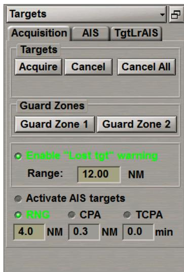
Use the **Range** input box to set the distance within which the **Lost target** warning will be generated when the ARPA or AIS loses a target. Beyond the set distance the lost targets are not at all displayed on the ECDIS task screen any more without warning.
