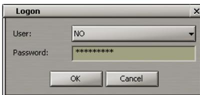
Enter the password for the appropriate access level. Press the **OK** button. The route will be protected from editing, and the letter “[P]” will be added to its name.
