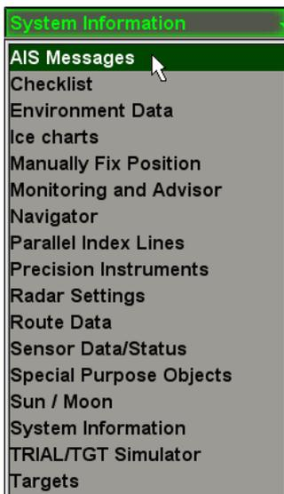
In the list which will open up, select the **AIS Messages** line and press the left trackball button.
