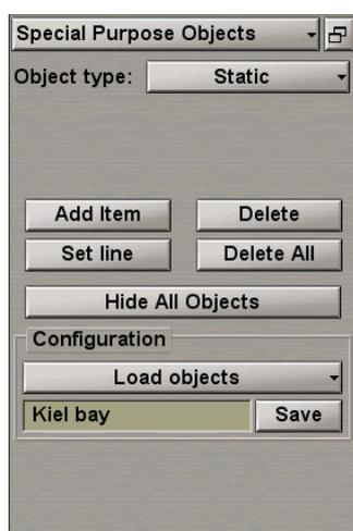
To save an SPO configuration, enter the configuration name in the input line of the **Configuration** group and press the **Save** button which will be enabled. SPO configuration files are accessible with the use of the Data Tool utility, in the **SPO objects** group of the **SPO objects** feature, and can be imported/exported from/to another PC.
