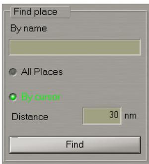
Press the **Find** button. Position the graphic cursors which will appear, on the point within the Chart panel which will be the centre of the area coverage circle.
