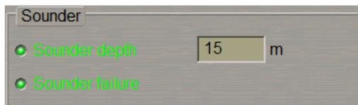
Use the **Sounder depth** line to enter the safety depth value from the echo sounder. Select the activated **Sounder depth** checkbox for turning on the alert generation as a depth smaller than the set one is detected.
