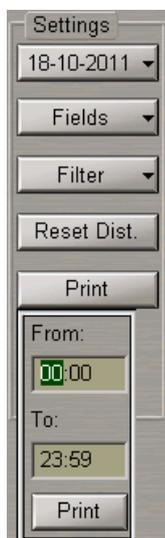
Use the **From** and **To** input boxes to set the time interval for the printout of the electronic system log book events, and press the **Print** button.
