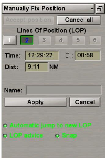
Enter the distance to the object in the **Dist** input box by using the trackball or keyboard. Press the left trackball button.
