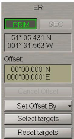
To monitor parameters of the ER mode, press the button with the name of the set display in the **Display Panel** window of the Control panel.
