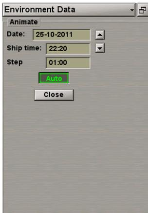
In the **Date** and **Ship time** input lines of the **Animate** group which will open up, enter the required viewing start date and time.
