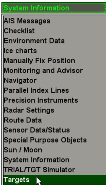
In the list which will open up, select the **Targets** line and press the left trackball button. Open the **AIS** page.
