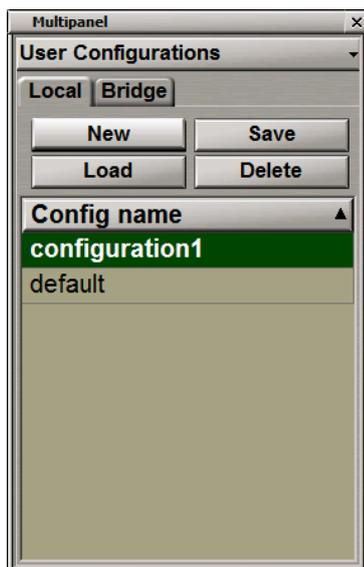
After the **New** button has been pressed, the current SW settings and the Graphic User Interface panels situation are saved automatically with the “Configuration X” name and are synchronized with all the running stations of the bridge (for information which is saved during the Local User Configuration creation see document *Multifunctional Display. Navi-Sailor 4000 ECDIS (v. 3.02.350). Functional Description, Chapter 3, section User Configurations*).
