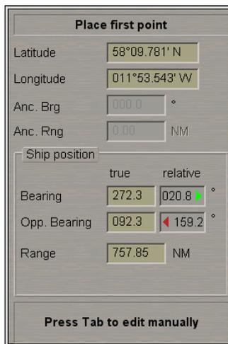
Set the cursor in the start point coordinates by moving the trackball, using the data in the **Place First Point** window, and press the left trackball button.
