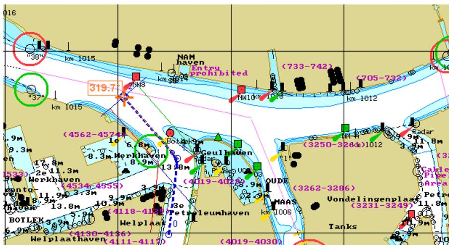
If it is necessary to set several waypoints, repeat the trackball moving and left button pressing operation as many times as there are WPT's required to be set.
