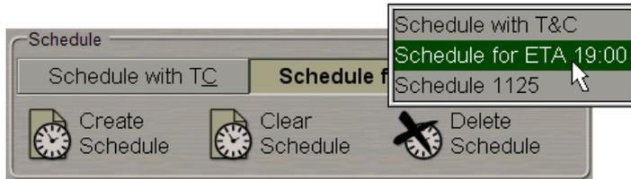
Select the schedule which should be deleted from the list, and press the left trackball button. In the window, which will appear, confirm the deleting.
