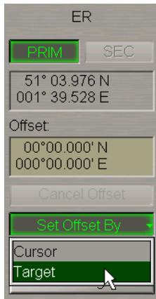
Position the acquisition marker which will appear on the required reference point.
