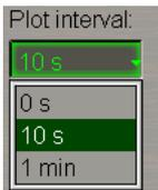
In the list which will open up, select the track plot interval and press the left trackball button.
