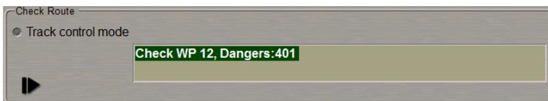
The route check will be interrupted. It can be resumed after the necessary time without exiting from the route checking mode. To do this, press the
