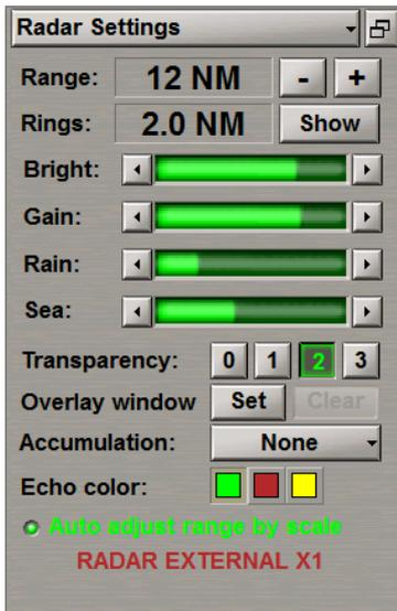
In the **Radar Settings** display which will open up, set the range scale. To do this, use the buttons to the right of the **Range** input box.
