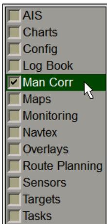
To turn on/off the display of updating objects on the ECDIS task screen press the button in the top left corner of the panel.
