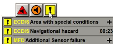
Category A alerts from the RADAR source can be acknowledged in the RADAR task (Navi-Radar 4000 application) only. Category A alerts from the ECDIS source can be acknowledged in the ECDIS task (Navi-Sailor 4000 application) only. Even if it is not permitted to acknowledge an alarm in the ECDIS or RADAR task, it will nonetheless be displayed in the task's alert list. An alert which cannot be acknowledged is shown with the or icons ("Can't be acknowledged"):
