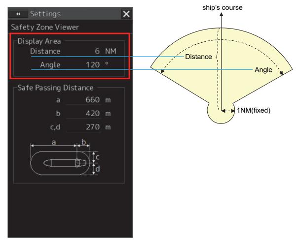
Note: [Angle] is the sum of the angles in the port and starboard directions with respect to your ship's course.
