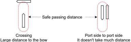
Therefore, by setting the CPA limit to a value smaller than the safe passing distance, it is possible to suppress unwanted CPA / TCPA alarms in congested waters and detect the danger of collision with "Need to Change Course" alarm. See 1.12.9 for details.
