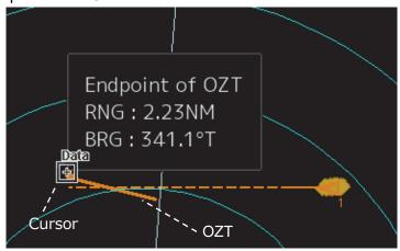
There are multiple targets and you don't sure which OZT belongs to which Target, you can change the color of the corresponding symbol and OZT by pointing the cursor over the OZT or AIS/TT symbol as shown in the figure below.
