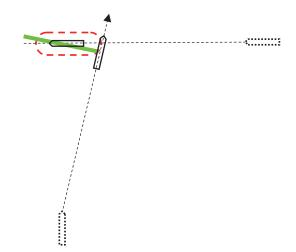
The safe passing distance can be changed in the menu. (Refer to 1.12.9) However, the OZT does not take into account the size of your ship and calculates it based on the ship's CCRP position. If the ship is a large vessel, it is advisable to set a large safe passing distance with a margin or to avoid the other ship so that it is sufficiently far from the OZT.
