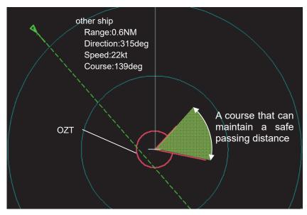
Your ship will not collide with the other ship that is faster than your ship and is moving away from your ship. Therefore, OZT does not exist on such a ship. A ship that does not display OZT can be judged to have a relatively low collision risk.
