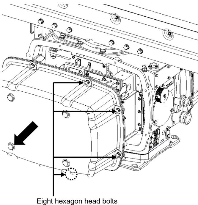
The magnetron is mounted on the left side (port side) of the radar antenna. Remove the left side cover.
