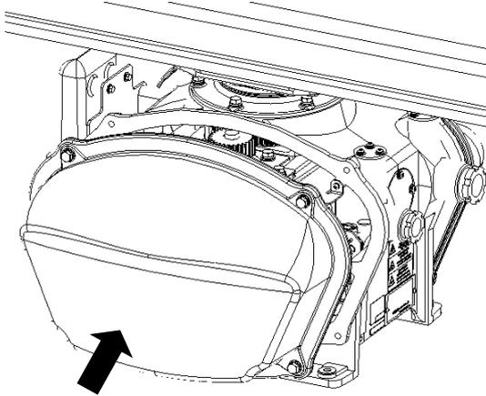
Before installing the cover on the radar antenna, check to confirm that there are no deformations, cracks or other abnormalities in the packing of the cover.
