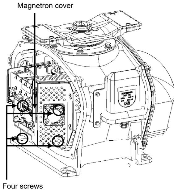
Loosen the screws (M4×10) at four positions to remove the magnetron cover.
