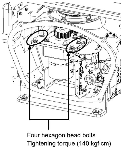
Install the motor in the radar antenna.
