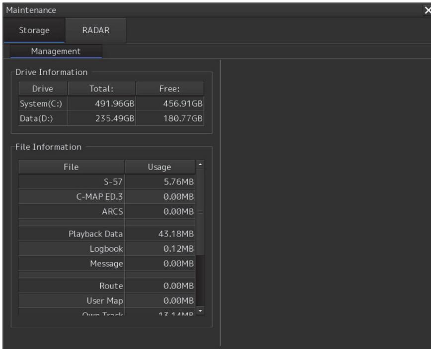
The total storage capacity and free space on each of the drives (C and D) are displayed in the [Drive Information] list. The capacity of each of the files stored on the drives is displayed in the [File Information] list. The files managed by File Manager are applicable.
