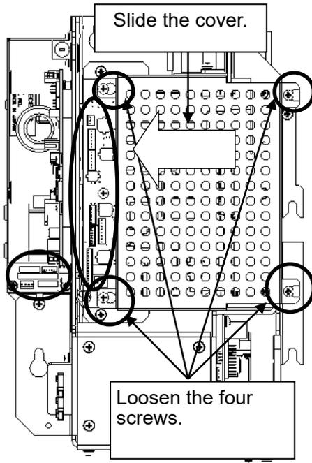
Loosen the screws (four M4 screws), remove the transmitter-receiver unit cover, and remove the cables connected to the transmitter-receiver unit (ten cables). Slide the cover of the transmitter-receiver unit to remove it.
