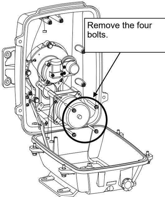
Remove the hexagon bolts (M6, at 4 places) and then remove the motor.
