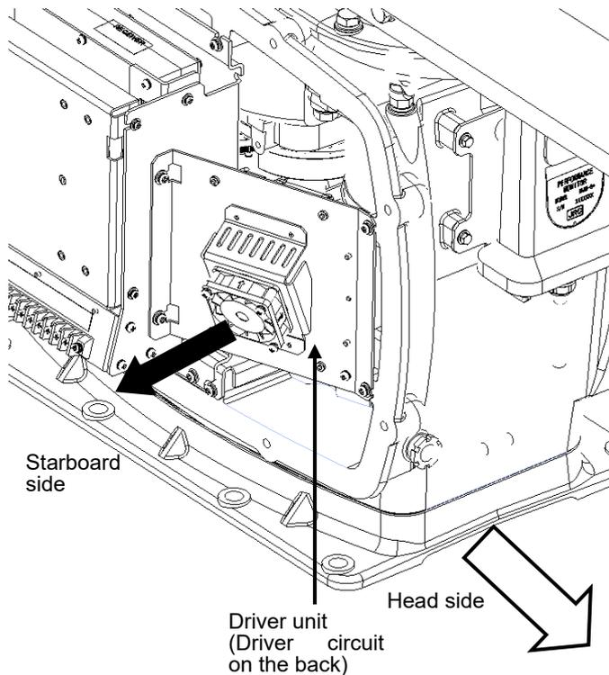
The motor driver unit is located on the right side (starboard side).
