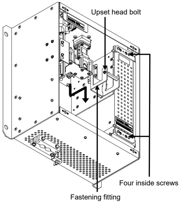
Loosen the upset head bolt (M4×12) and slide down the fastening fitting to remove it.
