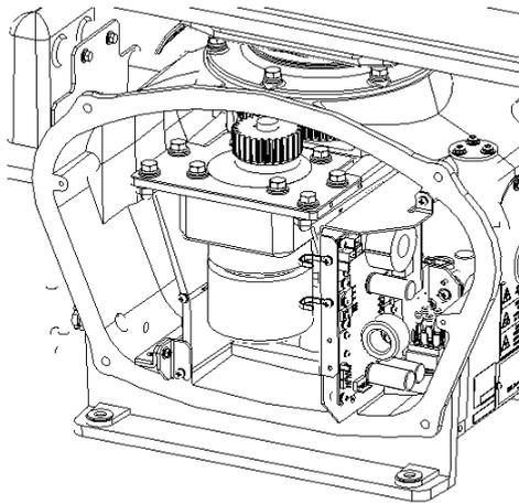
Reconnect the cables to the motor control power circuit.
