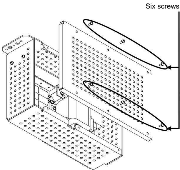
Loosen the screws (M4×10) at six positions and remove the modulator cover.
