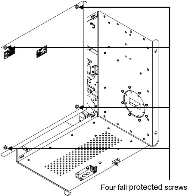
Loosen the four screws designed to be protected from falling out, and remove the cover.
