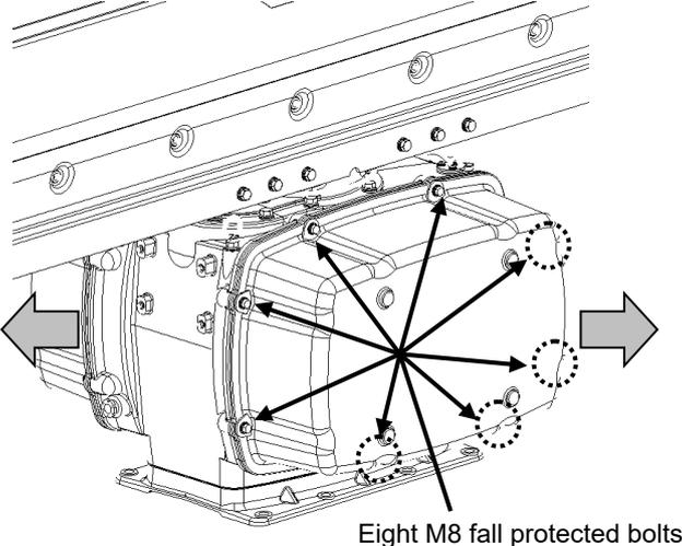
**!** When replacing a motor, ensure that the safety switch of the radar antenna is turned Off prior to commencing the replacement work.
