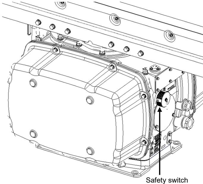
**!** When replacing a magnetron, ensure that the safety switch of the radar antenna is turned Off prior to commencing the replacement work.
