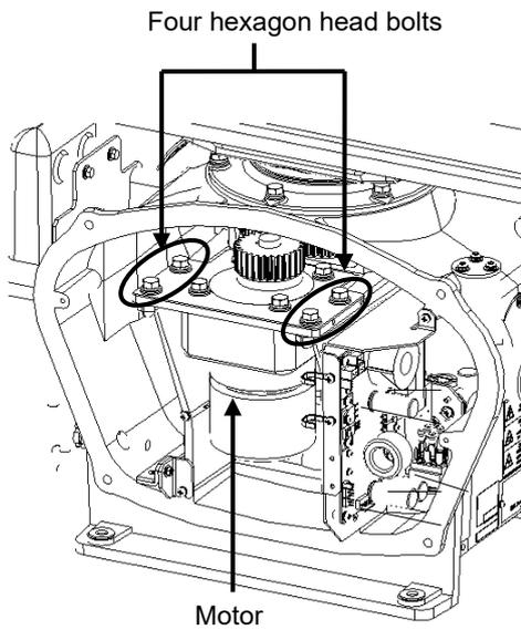
The motor is secured in place with hexagon head bolts (M8×20, SW + W assembled) at four positions.
