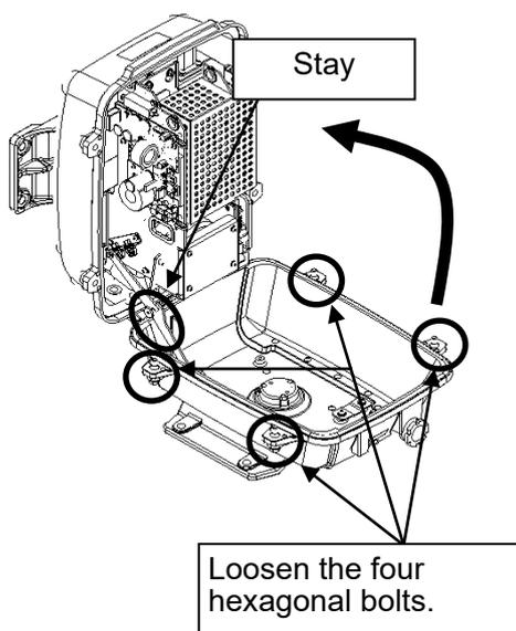
The top cover is fixed with 4 hexagonal bolts (M8 captive screw).
