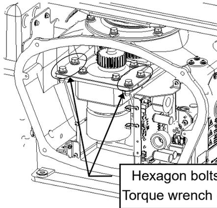
Place the motor in the antenna.
