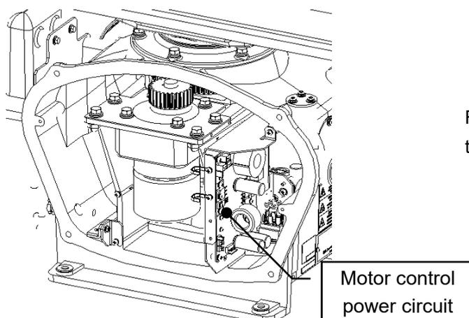
Remove the motor cable connected to the motor control power circuit.
