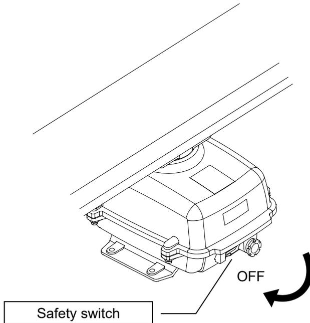
**!** When replacing a motor, make sure to first turn off the antenna safety switch.
