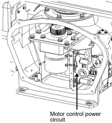
Detach the motor cables connected to the motor control power circuit.
