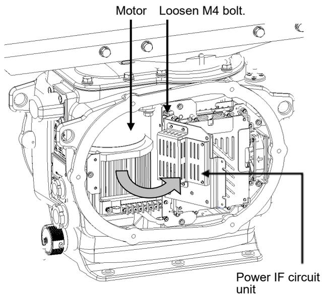
Loosen the M4 bolt and fix the power IF circuit unit with the unit open.
