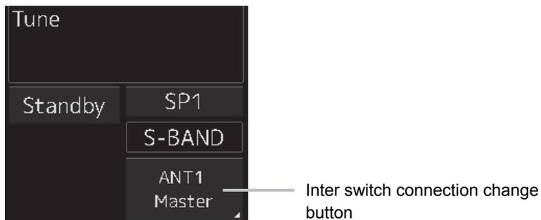
The name of the connected radar antenna is displayed in the upper part.
