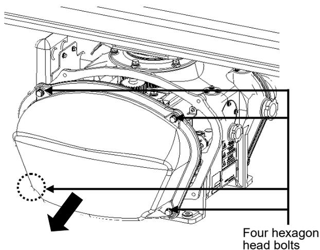
The motor is mounted on the left side (port side) of the radar antenna. Remove the left side cover.
