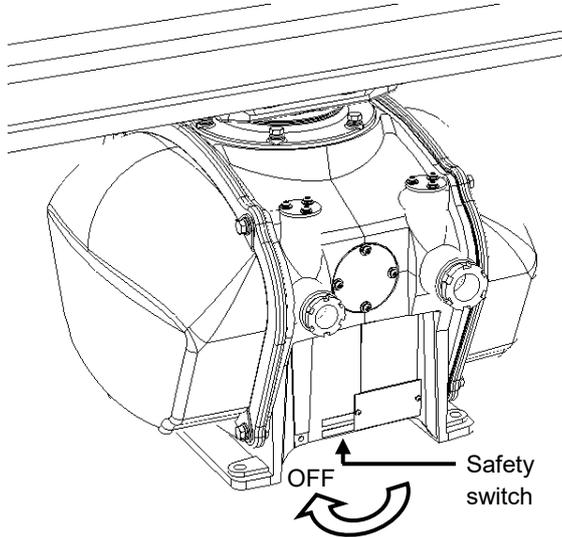
**!** When replacing a magnetron, turn Off the safety switch of the radar antenna.
