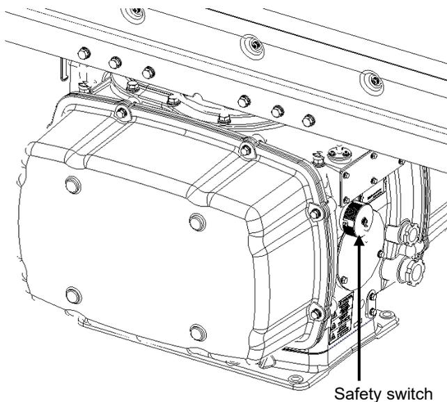
**!** When replacing a motor, ensure that the safety switch of the radar antenna is turned Off prior to commencing the replacement work.
