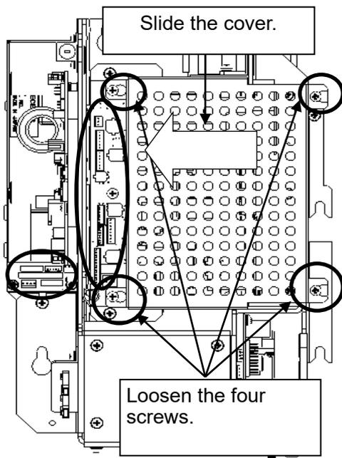
Loosen the screws (four M4 screws), remove the transmitter-receiver unit cover, and remove the cables connected to the transmitter-receiver unit (ten cables). Slide the cover of the transmitter-receiver unit to remove it.
