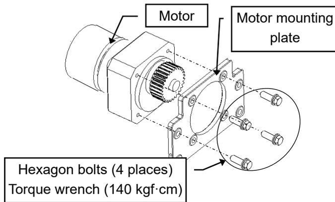
Attach the mounting plate to the new motor.
