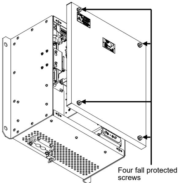
Loosen the screws designed to be protected from falling out at four positions, and remove the cover.
