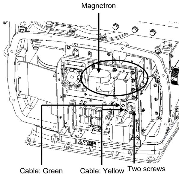
To detach the cables to which the magnetron is connected, remove the two screws (M4×12) holding the cables.
