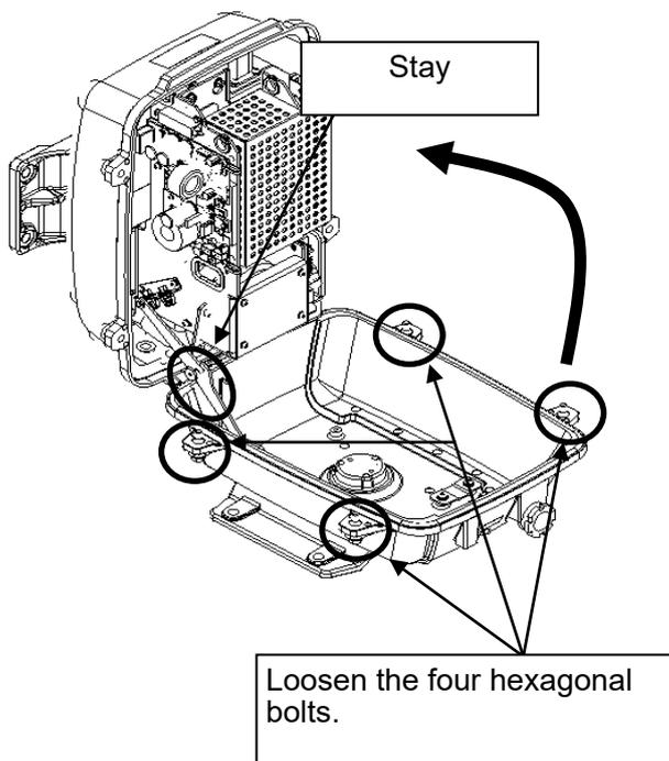
The top cover is fixed with 4 hexagonal bolts (M8 captive screw).
