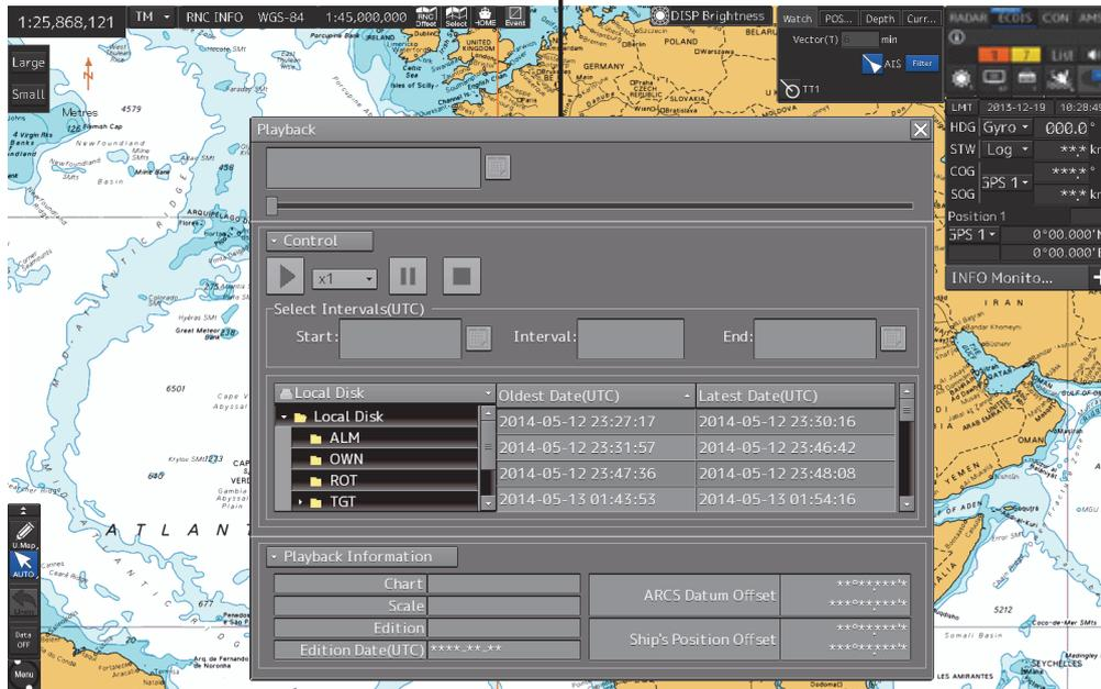
The playback controller can move to any position on the Playback dialog box; however, it cannot be minimized.
