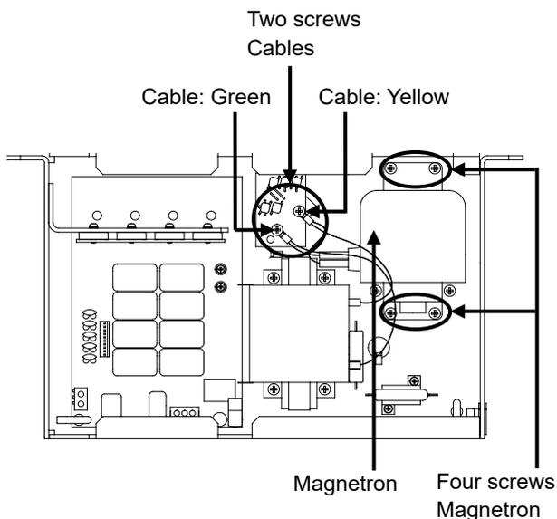
Remove the screws (M4×12) holding the cables at two positions, and detach the cables.
