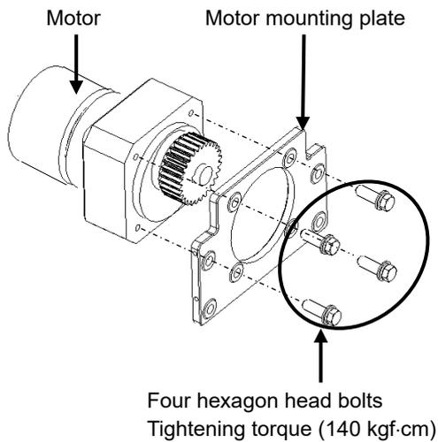
Set a mounting plate on a replacement motor.
