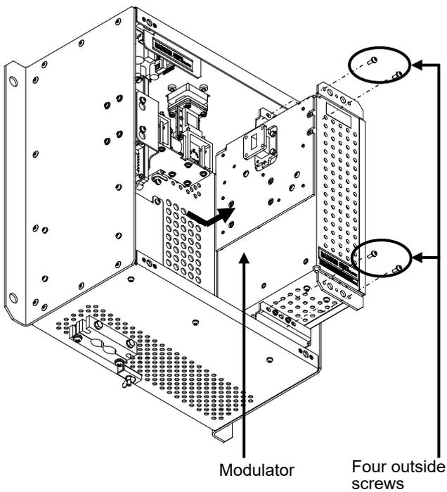
Loosen the outside screws (M4×12) at four positions and slide the modulator to the right to remove it.
