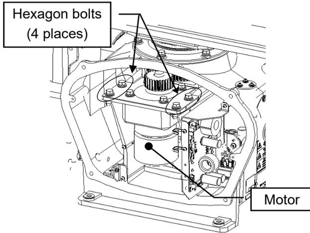
The motor is fixed with 4 hexagon bolts (M8 x 20 SW W, embedded type).
