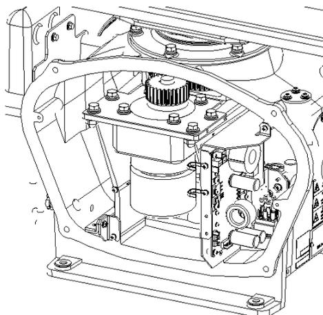
Connect each cable back to its original position on the motor control power circuit.
