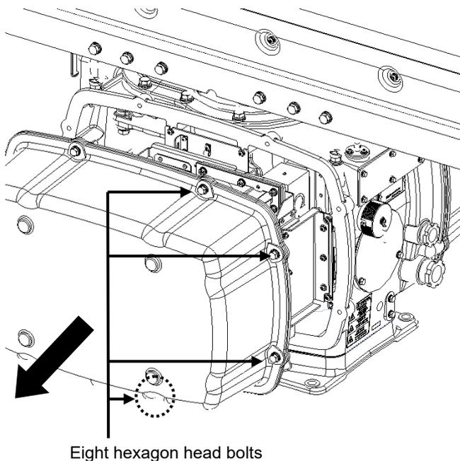
The motor is mounted on the front side (head side) of the radar antenna. Both left and right side covers need to be removed to carry out the motor replacement work.
