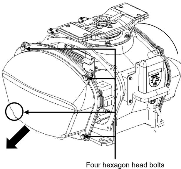
The magnetron is mounted on the right side (starboard side) of the radar antenna. Remove the right side cover.
