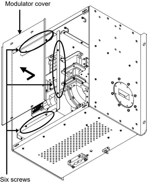
Loosen the screws (M4×12) at six positions and slide the modulator cover to the right to remove it.
