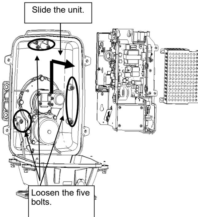
Loosen the bolts (five M5 bolts) and remove the transmitter-receiver unit. Slide the transmitter-receiver unit upward to remove it.
