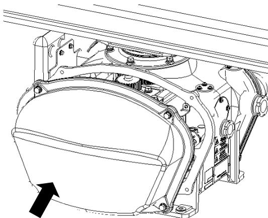
Before attaching the cover to the antenna, make sure that the gasket of the cover is not deformed or cracked. Also, remove any dust attached to the gasket.
