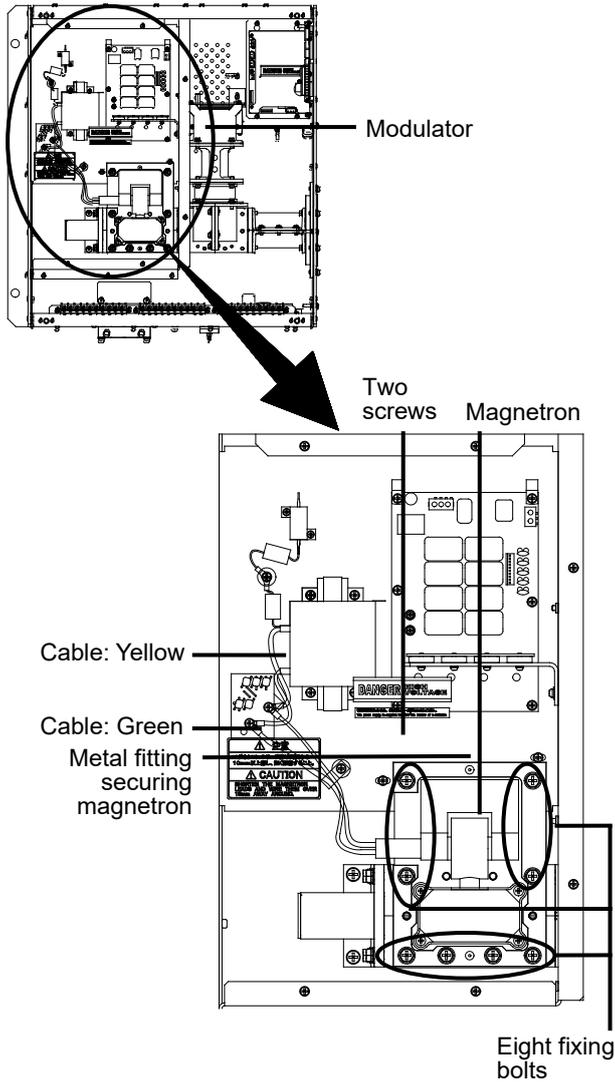
Remove the screws (M4×12) holding the cables at two positions, and detach the cables.
