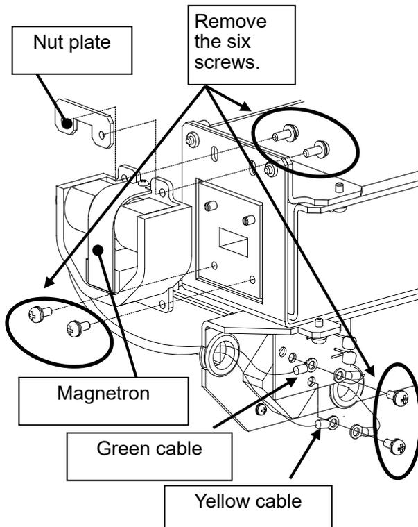
Remove the screws (six M4 screws) holding the magnetron in place and replace the magnetron.
