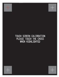
When the touch position and the reaction position are out of alignment, it can be corrected by performing calibration.
