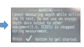
This function cannot completely identify the failure of the transducer. Use this as a guide to see when the transducer is operating normally.
