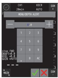
DEPTH ALERT the following menu will be displayed. Depth where the depth alert starts is set. and
