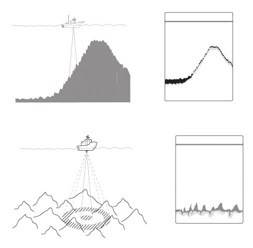
The echo of a seabed with abrupt slope is recorded as a lone difficult to see and less discriminative, since it tends to accompany with a false echo due to the side lobe and the inherent property of directivity.
