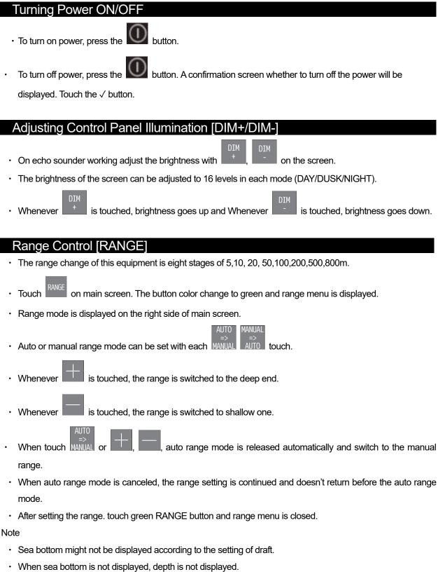
• Auto range automatically switches the range so that the bottom 3/5 of the range scale shows the sea bottom.
