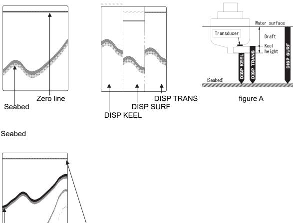
Zero line Third reflection of bottom Second reflection of bottom Seabed
