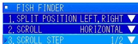
Turn the [MULTI] knob to select "3. SCROLL STEP". Press the [MULTI] knob to display the pulldown menu.
