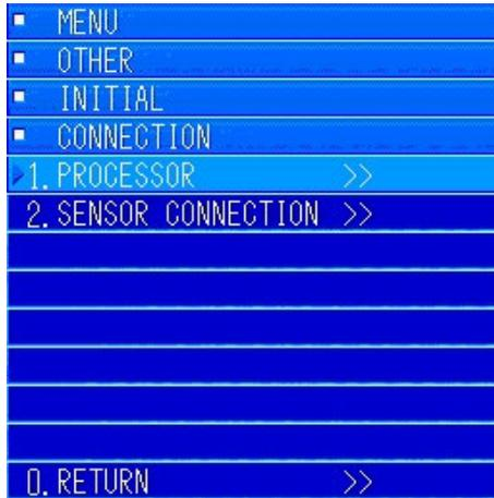
Open the "1. INITIAL" menu. Turn the [MULTI] knob to move to "3. CONNECTION", and then press the [MULTI] knob to open the submenu.
