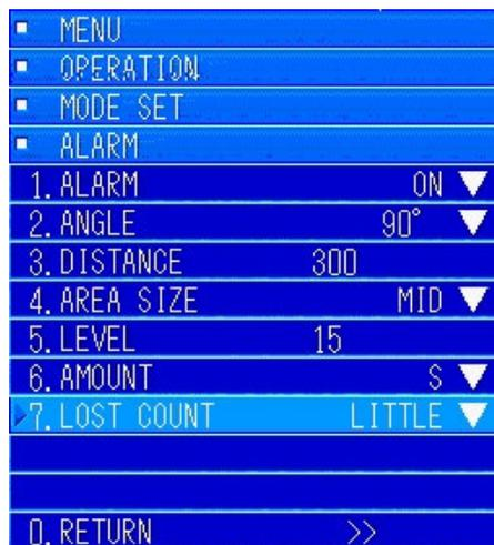
Use the [MULTI] knob to open the submenu for "ALARM" to do "ALARM" operations.
