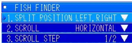
When the submenu is displayed, do the settings for items 1 through 3.
