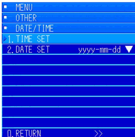
Move to "DATE/TIME". Press the [MULTI] knob to open the submenu. Turn the [MULTI] knob to move to "1. TIME SET" and a specialized menu opens. In the position you want to change, press the [MULTI] knob; press it until the white frame moves. After the frame moves, turn the [MULTI] knob to set a value. To finish, move the cursor to "SET" and press the [ENT] key to return to the menu.
