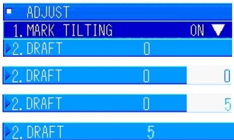
In the [6. ADJUST] menu, turn the [MULTI] knob to select "2. DRAFT". Press the [MULTI] knob to display the menu for inputting values.
