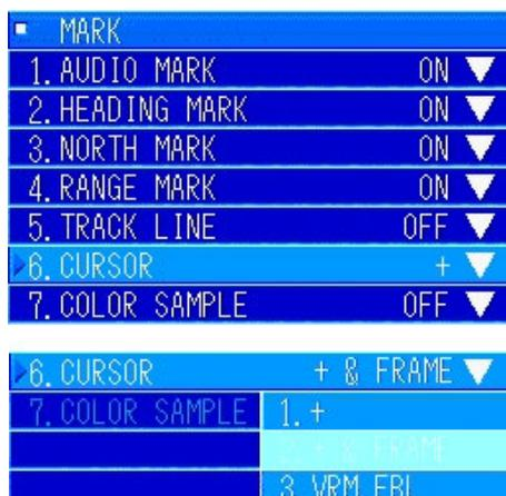
Turn the [MULTI] knob to select "6. CURSOR". Press the [MULTI] knob to display the pulldown menu.
