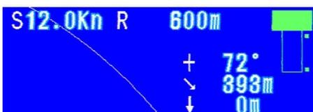
When the ship's speed falls below the set value, the ship's speed display changes to its normal color. Extension is now possible.
