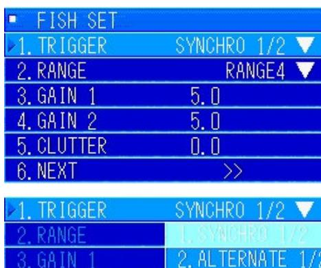
Turn the [MULTI] knob to select "1. TRIGGER". Press the [MULTI] knob to display the pull-down menu.
