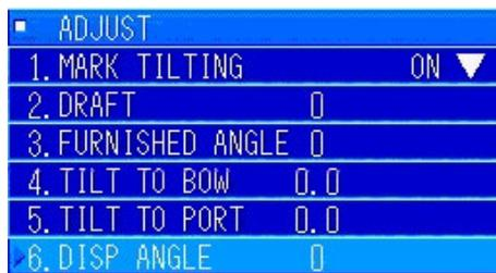
In the [6. ADJUST] menu, turn the [MULTI] knob to select "6. DISP ANGLE". Press the [MULTI] knob to display the menu for inputting values.
