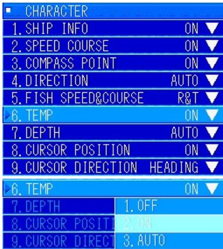
Turn the [MULTI] knob to select "6. TEMP". Press the [MULTI] knob to display the pulldown menu.
