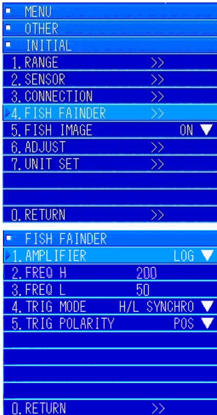
Open the "1. INITIAL" menu. Turn the [MULTI] knob to move to "4. FISH FINDER", and then press the [MULTI] knob to open the submenu.
