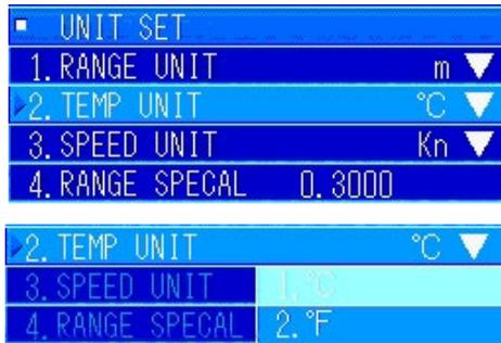
In the [7. UNIT SET] menu, turn the [MULTI] knob to select "2. TEMP UNIT". Press the [MULTI] knob to display the pulldown menu.
