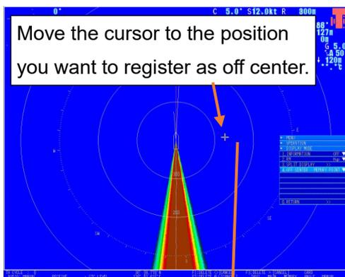
**Procedure to register off center and procedure to move off center**
