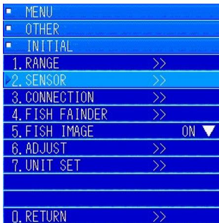
Open the "1. INITIAL" menu. Turn the [MULTI] knob to move to "2. SENSOR", and then press the [MULTI] knob to open the submenu.
