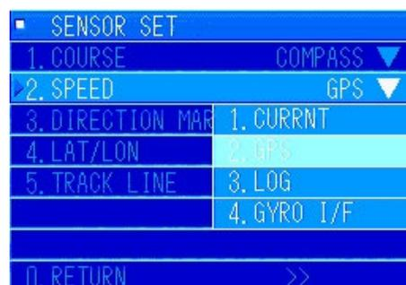
In the [SENSOR SET] menu, turn the [MULTI] knob to select "2. SPEED". Press the [MULTI] knob to display the pulldown menu.
