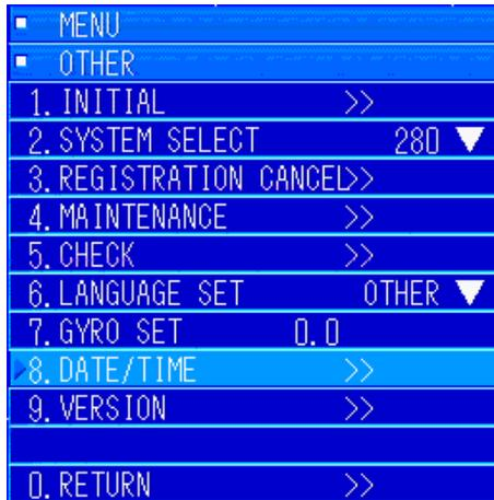
Press the [MENU] key to open the menu. Turn the [MULTI] knob to move to "9. OTHER". Press the [MULTI] knob to open the submenu. Turn the [MULTI] knob to move to "8. DATE/TIME". Press the [MULTI] knob to open the submenu and do time and date settings.
