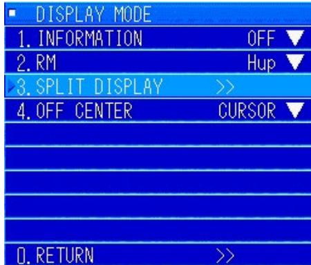
Turn the [MULTI] key to select "3. SPLIT DISPLAY". Press the [MULTI] knob to display the submenu, select either "1. AUDIO" or "2. F/F", and then set it.
