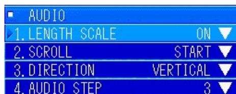
Turn the [MULTI] knob to select "1. LENGTH SCALE". Press the [MULTI] knob to display the pulldown menu.
