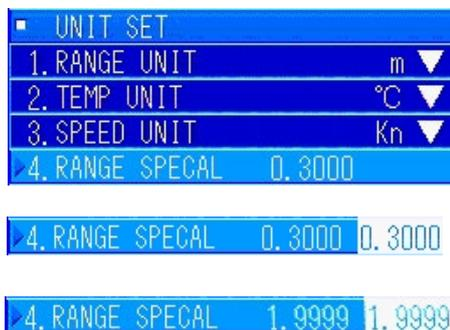
In the [7. UNIT SET] menu, turn the [MULTI] knob to select "4. RANGE SPECIAL". Press the [MULTI] knob to display the menu for inputting values.
