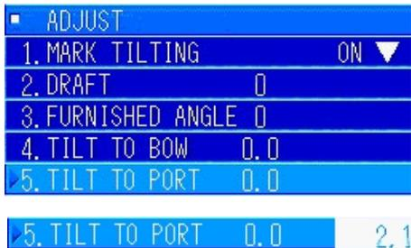
In the [6. ADJUST] menu, turn the [MULTI] knob to select "5. TILT TO PORT". Press the [MULTI] knob to show the display for inputting values.
