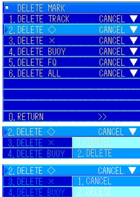
Follow the operations for deleting marks. Open the "DELETE MARK" menu. Turn the [MULTI] knob to select "2. DELETE ◇". Press the [MULTI] knob to display the pulldown menu.
