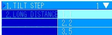
In the pulldown menu, "1. 1", "2. 2", or "3. 5" is set. For this product, we recommend "3. 5" according to the vertical beam width, when using automatic tilt.
