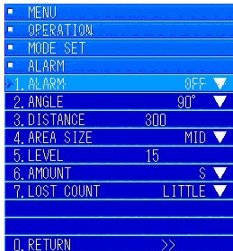
To turn the alarm function "On", turn the [MULTI] knob to move to "1. ALARM". Press the [MULTI] knob to display the pulldown menu, as shown in the diagram below.
