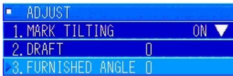
In the [6. ADJUST] menu, turn the [MULTI] knob to select "3. FURNISHED ANGLE". Press the [MULTI] knob to display the menu for inputting values.
