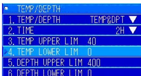
Turn the [MULTI] knob to select "4. TEMP LOWER LIM". Press the [MULTI] knob to display the menu for inputting values.
