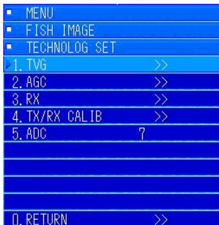
Move to the "TECHNOLOG SET" menu and turn the [MULTI] knob to move to "1.TVG". Press the [MULTI] knob to open the submenu.
