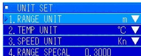
In the [7. UNIT SET] menu, turn the [MULTI] knob to select "1. RANGE UNIT". Press the [MULTI] knob to display the pulldown menu.
