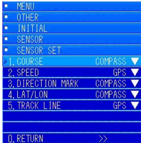
In the [SENSOR SETTINGS] menu, turn the [MULTI] knob to select "2. SENSOR SET". Press the [MULTI] knob to display the submenu.
