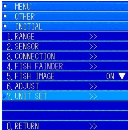
Open the "1. INITIAL" menu. Turn the [MULTI] knob to move to "7. UNIT SET", and then press the [MULTI] knob to open the submenu.
