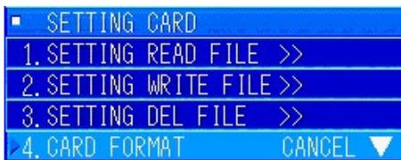
Open the submenu for "5. SETTING CARD", the same as in the previous section.
