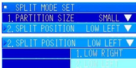
Turn the [MULTI] knob to select "2. SPLIT POSITION". Press the [MULTI] knob to display the pulldown menu.
