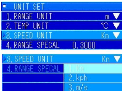
In the [7. UNIT SET] menu, turn the [MULTI] knob to select "3. SPEED UNIT". Press the [MULTI] knob to display the pulldown menu.
