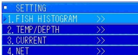
Press the [MULTI] knob to open the submenu. You can change the display settings from 1 to 4.
