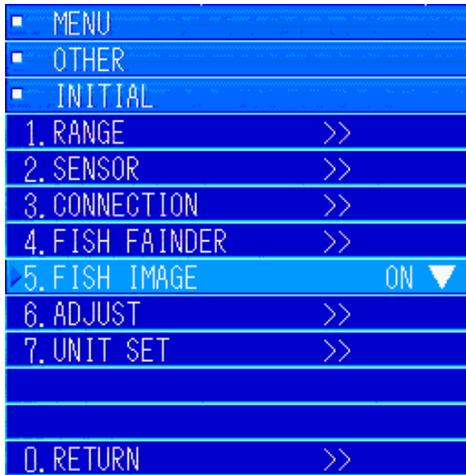
Open the "1. INITIAL" menu. Turn the [MULTI] knob to move to "5. FISH IMAGE", and then press the [MULTI] knob to open the pulldown menu.
