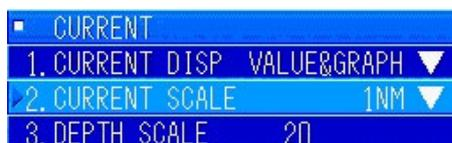
Turn the [MULTI] knob to select "2. CURRENT SCALE". Press the [MULTI] knob to display the pulldown menu.
