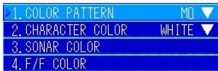
Turn the [MULTI] knob to select "1. COLOR PATTERN". Press the [MULTI] knob to display the pulldown menu.
