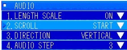
Turn the [MULTI] knob to select "2. SCROLL". Press the [MULTI] knob to display the pulldown menu.
