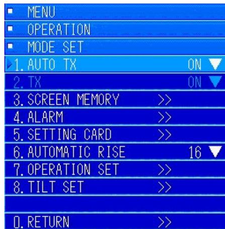
Turn the [MULTI] knob to move to "1. AUTO TX". Press the [MULTI] knob to display the pulldown menu.
