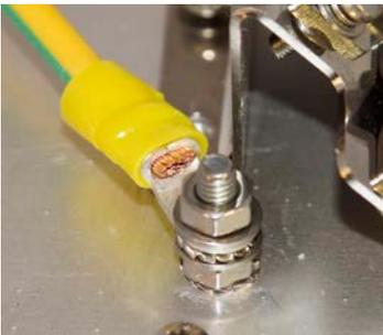
**Figure 6: Grounding Bolt**
