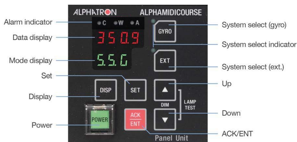
Figure: Operating Panel
