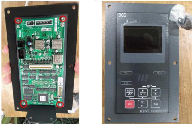
7. Connect delivered DGA 15 cable with connector in J71 socket on backside of DGC-01 Operation Panel and connect the other side of DGA15 cable to J71 socket inside the DGC-01 as example shown in below figure.
