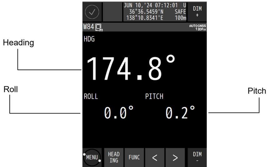
Sub Screen 2 (Ship's heading, heaving, roll, pitch, ROT)
