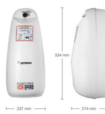
TCP/IP protocol (IEE802.3) 80 GB SSD (48 hr record) Operates 168 hr after activation Proteced up to 10 m depth 5 min 406/121.5 MHz EPIRB frequency Temperature: -20°C to 55 °C Power from NDV-1900/1950
