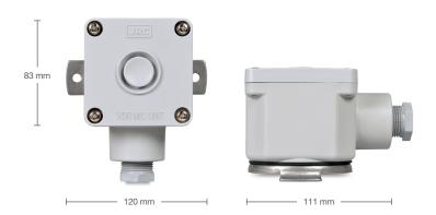
Wall mount installation Range receive radius 3.5m Built-in speaker for audio test Temperature: -25° to 55°C Protection rate: IP56 Compass safety distance 0.1m Power from NDV-1900
