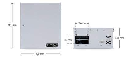
Up to 48 channel IEC61162 -1 (22ch), -2 (2ch), -450 (24 sensors) Microphone 12 ch (6 tracks) VHF 4 ch (2 tracks) Image 6 ch (ECDIS, X & S radar) 512GB SS drive (720hr record) Power 100V to 240V AC (230VA)
