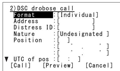
2. Select Address and press ENT, input the MMSI of the calling coast station.
