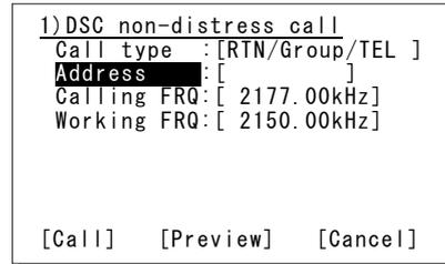
2. Input the Address, and frequency if required. And then press ENT on the Call to start sending the group call.
