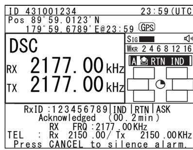
6. When requested the radiotelephone communication, start the communication with the handset.
