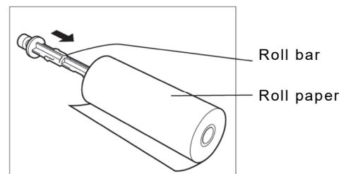
3. Pass the roll paper over the guide bar as shown in the figure at right.
