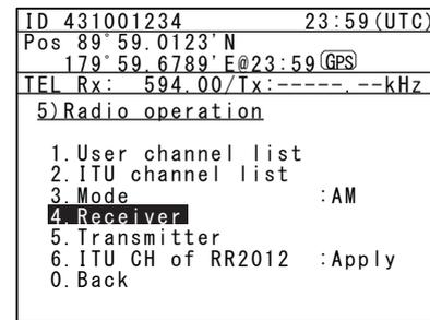
5. Press the **MENU** key twice to return to the status display and if required, input an AM broadcast frequency using the numeric keys. Then press ENT to receive the broadcast.
