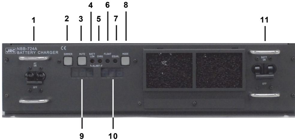
1. AC breaker ..... When turned on, enables to use the AC mains input.
