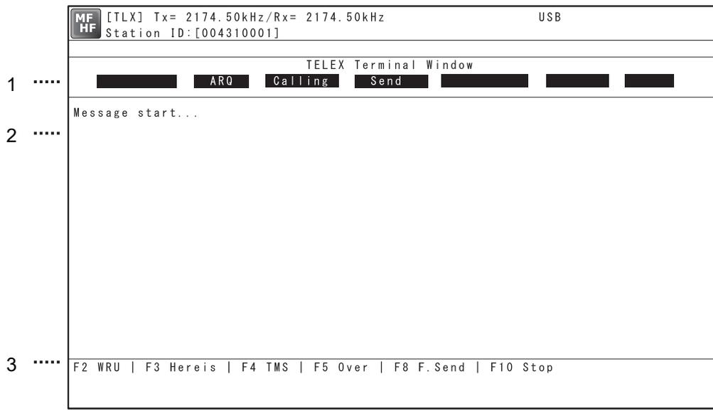
1. Indicates the operating condition of the telex communication from the left of each segment as follows.
