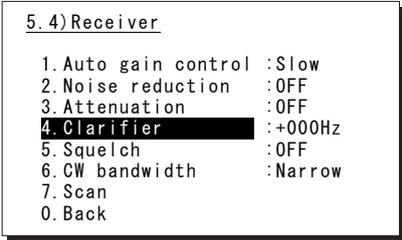
2. Press ENT to move the cursor to the right, then use the jog dial or numeric keypad to select a value in the range of -200 to +200 Hz.
