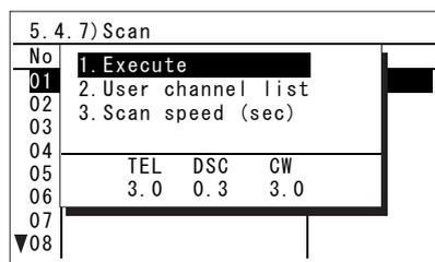
4. Select 1. Execute and press ENT, the screen at right is displayed and scanning starts.
