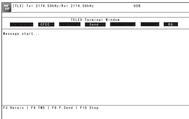
6. The characters typed with the keyboard can be transmitted in sequence. And all of the characters displayed on the screen are printed out on the printer.
