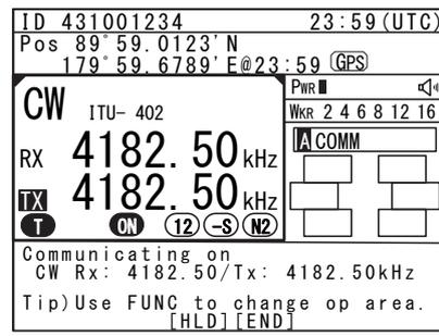
7. Communicate in CW mode using the CW keyer connected to the KEY jack on the controller as shown in the figure to the right.
