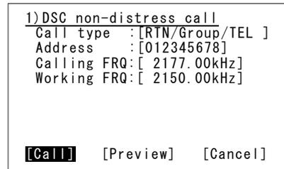
3. After finishing the transmission, the working frequency is set immediately.
