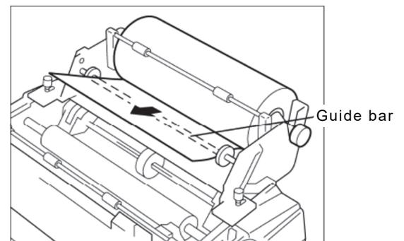
4. Pull the friction lever towards the front, and insert the leading edge of the paper into the rear of the platen. Then, return the friction lever to the back, and turn the paper feed knob to feed the paper out.
