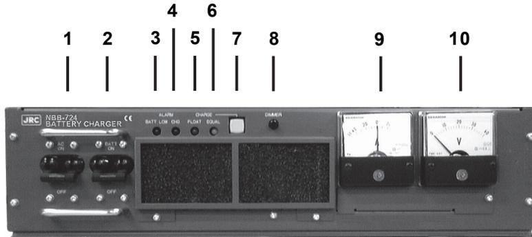
1. AC breaker ..... When turned on, enables to use the AC mains input.
