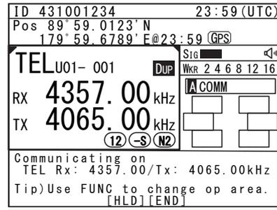
2. Pressing ENT causes the channel group number to blink so a channel group can be input.
