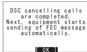
4. According to the guidance on the screen, broadcast to cancel the distress alert in TEL mode.
