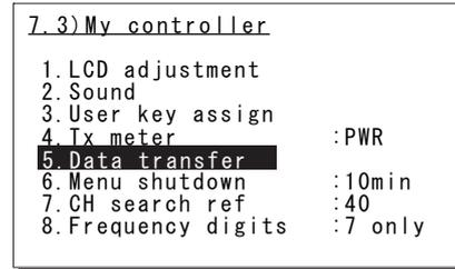
2. Move the cursor to 5. Data transfer with the numeric keypad or jog dial and press ENT.
