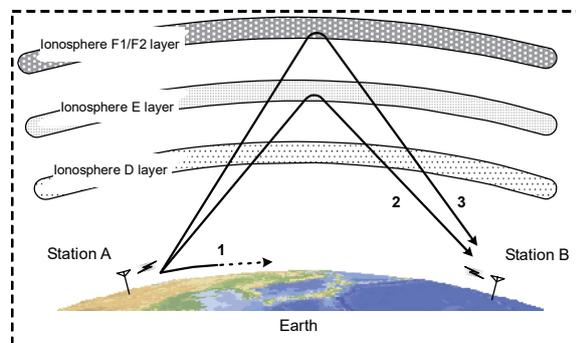
The available range of frequencies for communication depends upon the radio wave propagation characteristics of the ionosphere. They will also change dramatically depending on the position and distance from the station, the season, the time, and the sunspot number (approx. 0 to 250) which changes every 11 years<sup>7</sup>.
