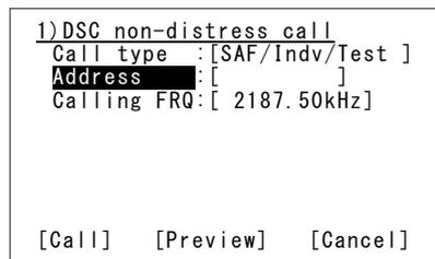
2. Press ENT on the Call to start sending the safety test call.
