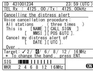
5. When the cancelling procedure is completed on every frequency, displays the operating screen as shown at right and finishes the distress mode.
