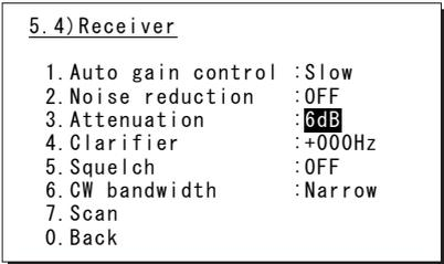
**Note** The same settings can be done by pressing and holding the **FUNC** key and the **4ATT** key at the same time.
