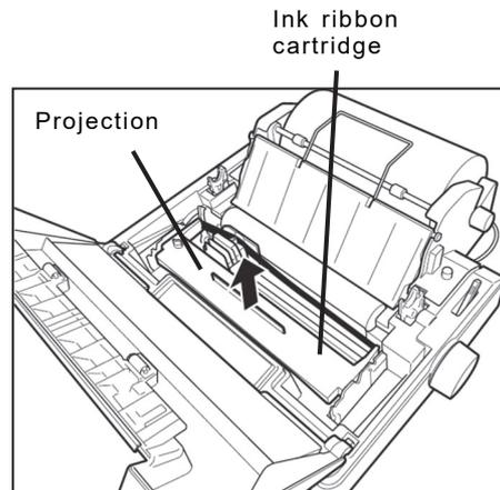
2. Using the knob on the new cartridge make the ribbon taut. Then manually move the print head to the left edge, and attach the ribbon with such a pen so that it is between the ribbon mask and print head.
