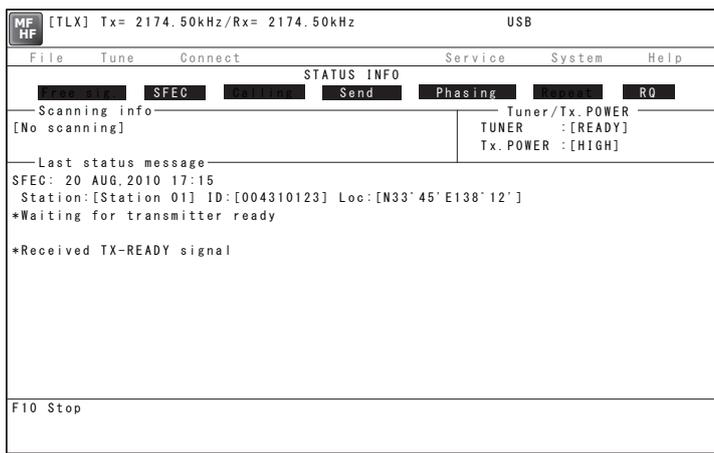
6. After sending the phasing signal followed by the SELCAL number, the message sending using the SFEC mode will be available.
