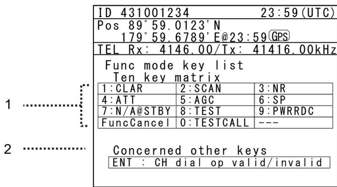
1. Indicates the enabled number key and its function when the FUNC key is pressed in the status display. Pressing the number keys here operates the function for that key as shown at the right.
