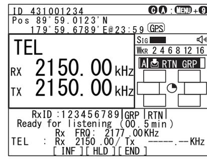
**Note** When receiving the group call where the FEC is specified, the telex mode is set to the equipment. Then receive the telex broadcasting with the data terminal.
