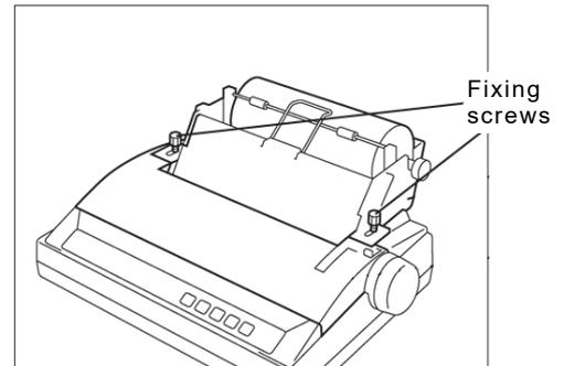
2. Pass the roll bar through the roll paper, and install the roll paper onto the roll paper stand paying attention to its orientation.
