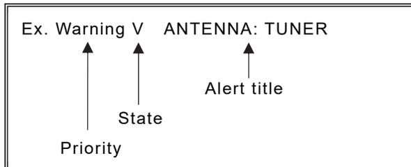
If ▲ or ▼ mark is indicated on the left edge, there are other alerts hidden outside the screen. Hold down the **PWR CONT** key and turn the jog dial to display the hidden alert in a single operation.
