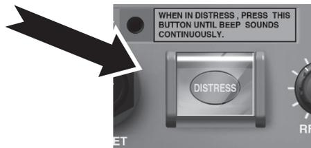
2. Press and hold the **DISTRESS** key for 4 seconds to send the distress alert. When the countdown is finished the screen below on the right is displayed, and after antenna tuning the distress alerts are transmitted.
