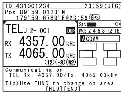
3. After inputting a group number, pressing ENT causes the channel number to blink so a user channel can be input.
