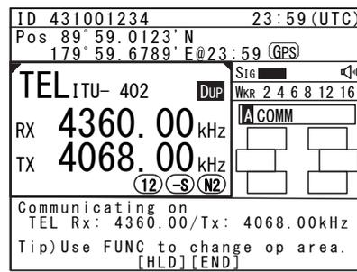
2. Input the channel by using the numeric keypad.
