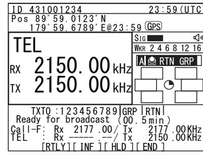
**Note** After completing the group call where the FEC is specified, the telex mode is set to the equipment. Then the telex communication can be started with the data terminal.
