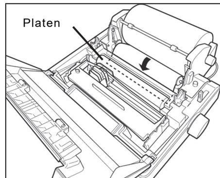
5. Restore the roll paper cover and the roll support cover as shown at right and close the printer cover.
