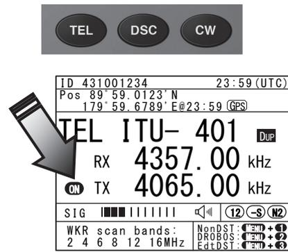
3. Set the frequency for making calls in radiotelephone mode.
