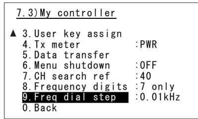
**5.3.9 Setting the frequency step width due to the jog dial**
