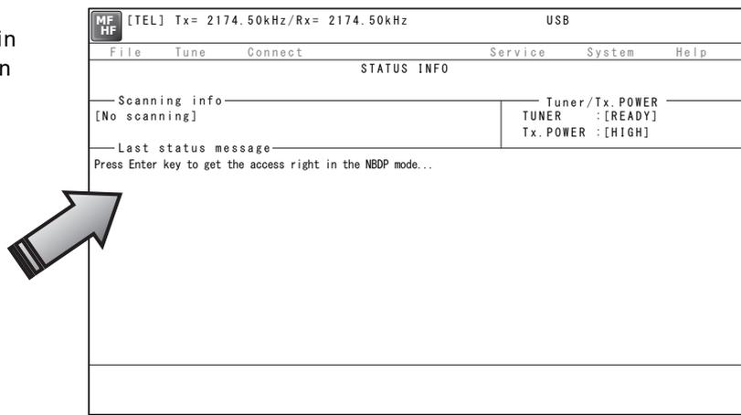
2. After checking the USB mark indicating on the top of the display of the data terminal, select File from the main menu and the objective dropdown menu.
