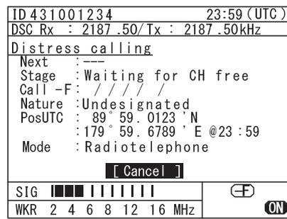
4. The equipment stays in distress mode until acknowledgement is received or the distress alert cancelling procedure is complete.
