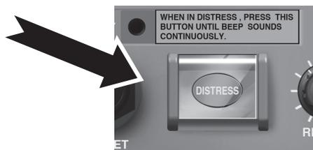
10. Press and hold the **DISTRESS** key for 4 seconds until the countdown is completed.
