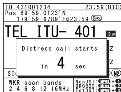
3. After the antenna is tuned, the distress alert is sent.
