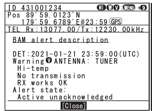
2. To display the BAM alert description, turn the jog dial to select the alert, then press ENT.
