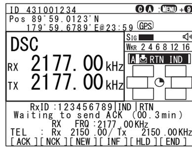
3. Press **FUNC** key or ENT to move the focused screen to the operation control screen and select the option to handle the procedure.
