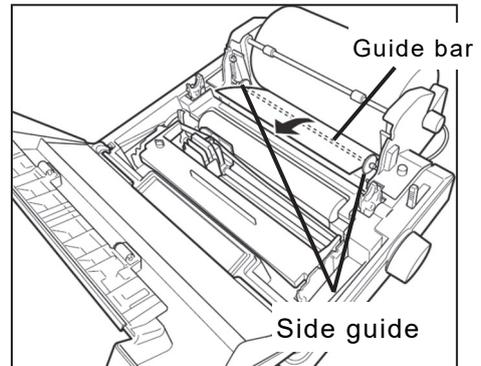
4. Insert the leading edge of the paper into the rear of the platen. Then turn the paper feed knob to feed the paper out and adjust the direction.
