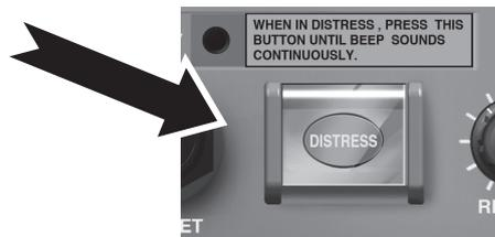
2. Press and hold the **DISTRESS** key for 4 seconds until the countdown is completed.
