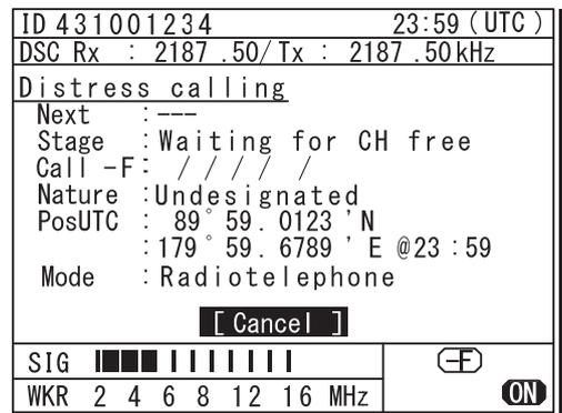
3. After sending the distress alert, wait for an acknowledgement. The radiotelephone can be used to communicate even while waiting for an acknowledgement on the screen below left. When an acknowledgement is received, press the **CANCEL** key or ENT to cancel the alert on the below right screen, and communicate with the station. Unless an acknowledgement is received or the distress alert is cancelled manually, the equipment repeats the distress alert every 3.5 to 4.5 minutes.
