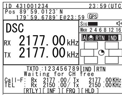
5. When receiving the acknowledgement the ALM lamp starts blinking, and the receiving alert starts sounding.
