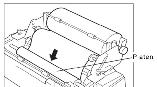
5. Lift the paper load lever up to hold down paper fed out of the platen.
