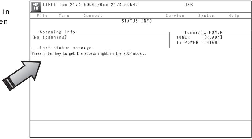
2. On the main menu and the dropdown menu, select System → NBDP setup with Enter key.
