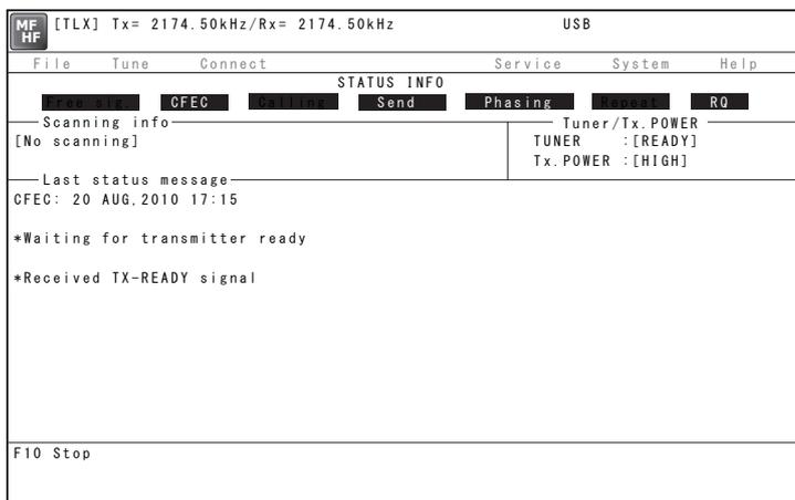
5. After sending the phasing signal for about 15 seconds, the message sending using the CFEC mode will be available.
