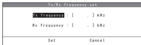
3. Input the receiving frequency of the CFEC broadcasting, and press Enter key.
