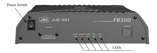
Fig.4.1.3a Power switch and LEDs of Main unit
