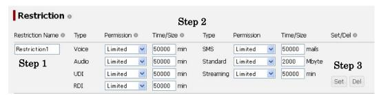
Fig. 6.5.4.3a Usage Restriction (Restriction Setting) Screen
