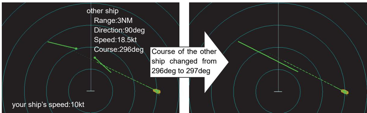
When the distance to the other ship is so close that there is little safe course to avoid it, the OZT may be displayed in an arc as shown below. This indicates that the only way to maintain a safe passing distance from the other ship is to proceed to a course without an arc.
