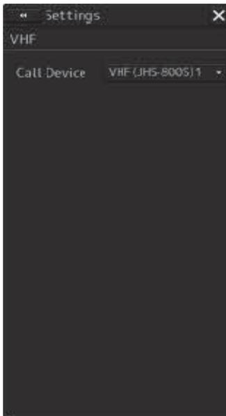
**4 Select JHS-800S on the [Call Device] combo box for VHF communication.**
