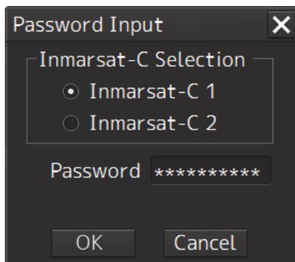
**3 When two units of JUE-87 are installed, select a terminal by clicking on the [Inmarsat-C1] or [Inmarsat-C2] button.**
