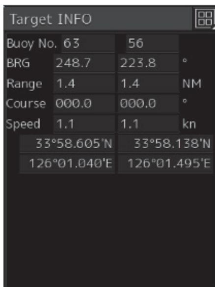
Right click on the GPS buoy symbol and select **Property...** from the context menu to display the properties of the target symbol.
