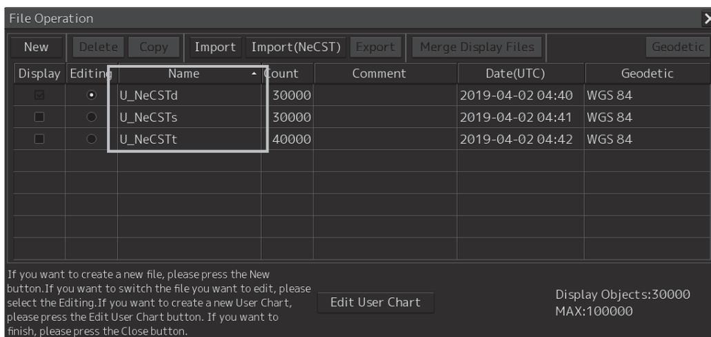
Also, A file name is saved the following according to the type of data that created on the J-Marine NeCST.
