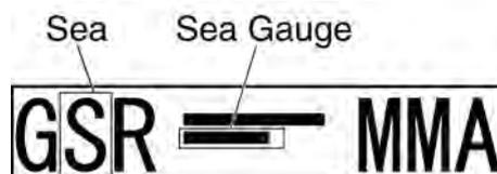
When turning the [SEA] control, the sea clutter control indication is stretched or shrunk.
