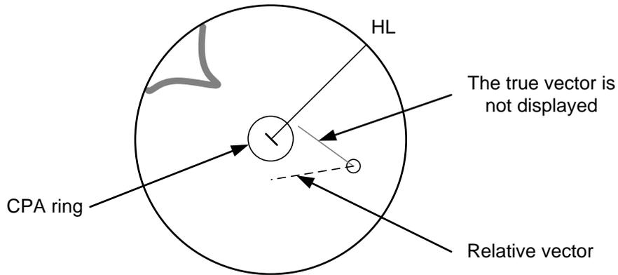
Therefore, the TRUE/REL mode shall optionally be used for the purpose of observation: the TRUE vector mode for grasping the true aspect of a target, and the REL vector mode for grasping a target's closest point of approach (CPA).
