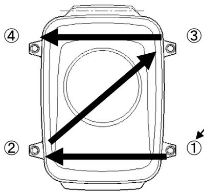
NKE-2062 Cover Bolt Tightening Procedure
