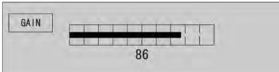
The sensitivity adjustment screen appears when turning the [GAIN] control.
