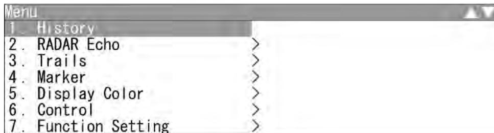
Select one of the menu items with ">" mark, then press the [ENT] key or the cursor key (right) to display the submenu.
