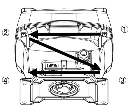
NKE-2063A/HS/AHS Cover Bolt Tightening Procedure
