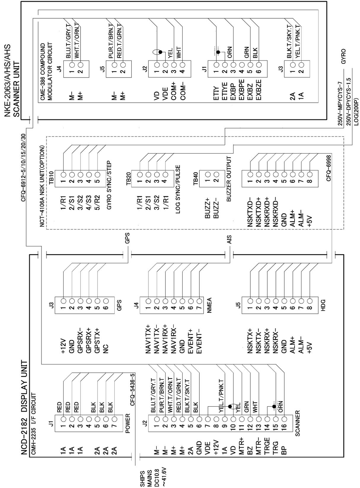
Fig. A16 JMA-3340-4/4HS/6/6HS INTERCONNECTION DIAGRAM
