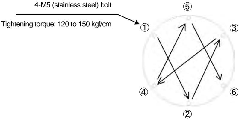
NKE-2043 Cover Bolt Tightening Procedure
