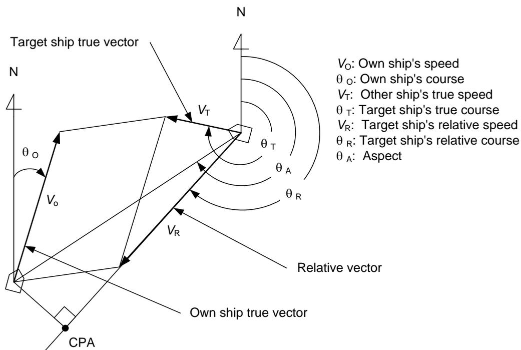
■ Radar and Collision Avoidance
