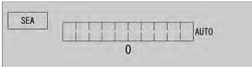
The sea clutter suppression adjustment screen appears when turning the [SEA] control. Sea clutter suppression can be adjusted between 0 and 100.
