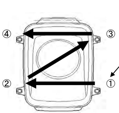
NKE-2103-4/4HS/6/6HS Cover Bolt Tightening Procedure
