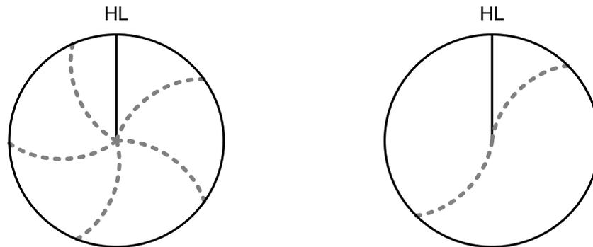
If radar equipment causing an interference pattern and this radar are of the same model, their transmitting repetition frequency is nearly the same. As a result, interference patterns may be displayed concentrically.
