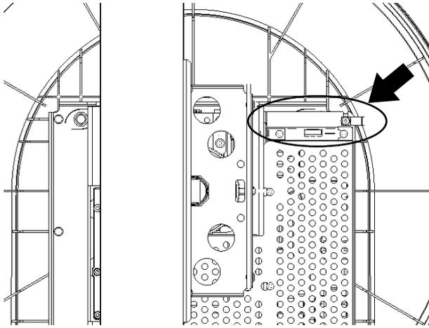
**3 Remove the motor cable, the receiver cable and the sensor cable.**
