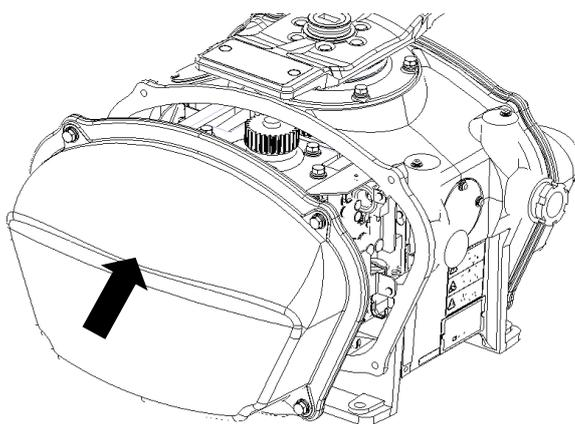
Before mounting the cover on the radar antenna, confirm that there are no abnormalities such as deformation and crack on the cover packing.
