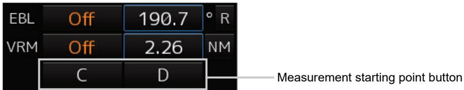
Each time this button is clicked on, the measurement starting point switches in the order of blank field → [C] → [D] → blank field and so on.
