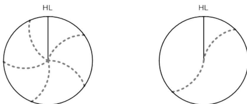
If radar equipment causing an interference pattern and this equipment are of the same model, their transmitting repetition frequency is nearly the same. As a result, interference patterns may be displayed concentrically.
