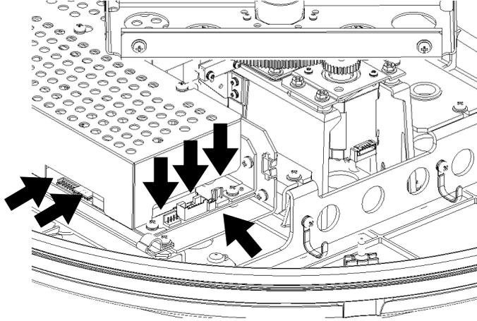
After connecting all cables, check the cables not to interfere the antenna rotation.
