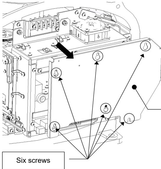
Remove the front cover from the transmitter-receiver unit.
