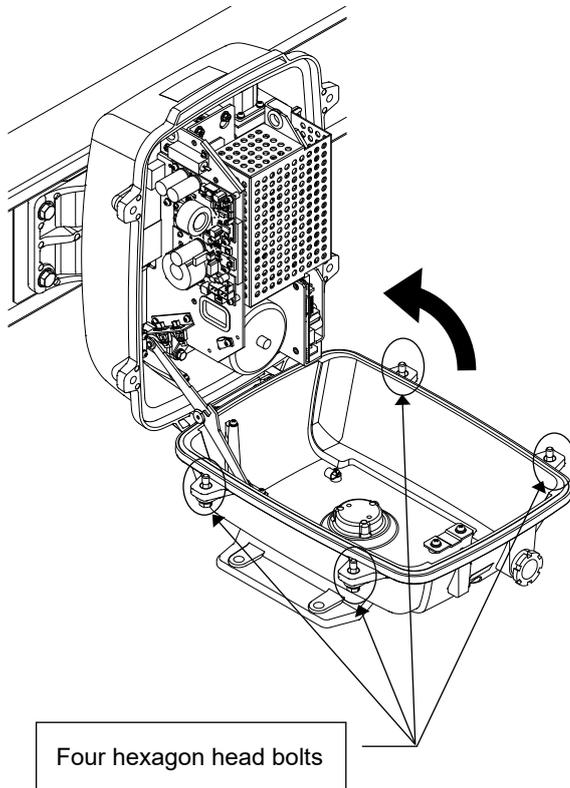
The upper cover is secured in place with hexagon head bolts (M8, designed to be protected from falling out) at four positions.
