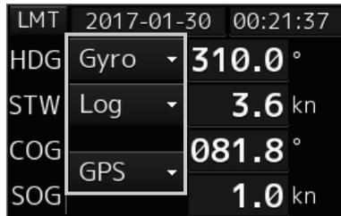
Select the sensor source in the [Source] combo box. The following sensor sources can be selected.
