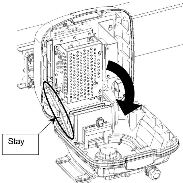
If any hexagonal bolt is not tightened enough or is loosened, the waterproof performance may be deteriorated. Be sure to tighten all bolts with specified torque (120 to 150kgf·cm).
