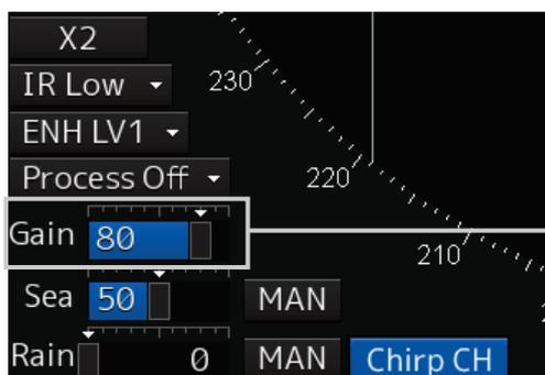
[Gain] (reception gain adjustment) slider
