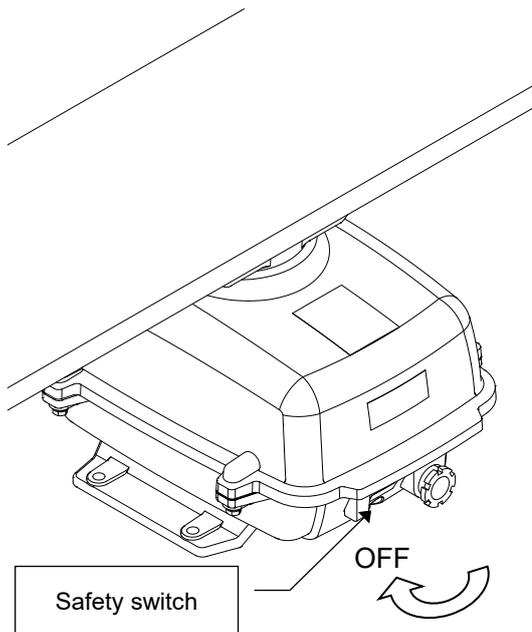
**⚠** When replacing a motor, ensure that the safety switch of the radar antenna is turned Off prior to commencing the replacement work.
