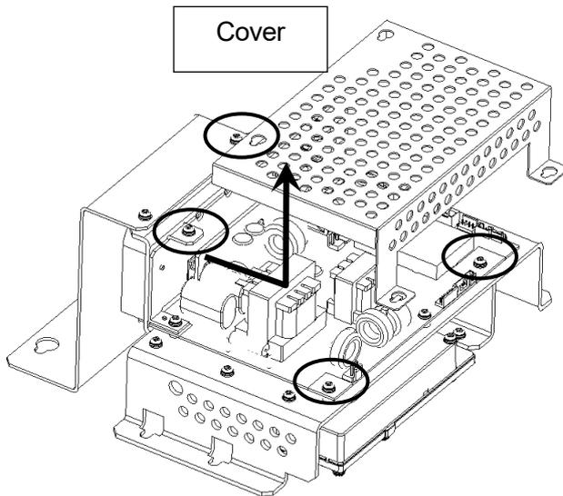
**5 Remove the support plate of the transceiver unit.**
