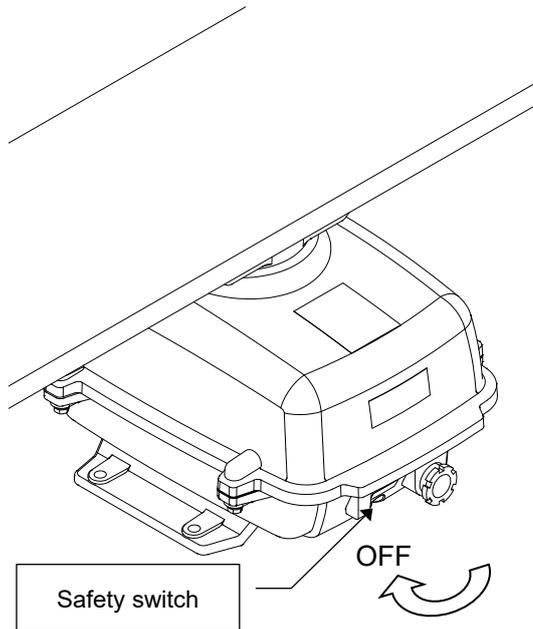
**⚠** When replacing a magnetron, ensure that the safety switch of the radar antenna is turned Off prior to commencing the replacement work.
