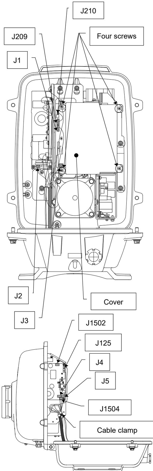
Loosen four screws (M4×12).
