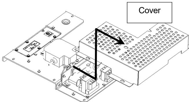
6 **Remove the magnetron cable.**
