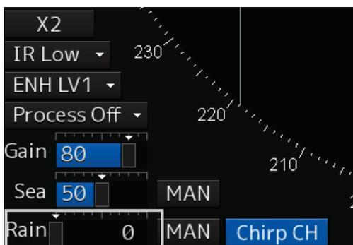
[Rain] (rain/snow clutter adjustment) slider
