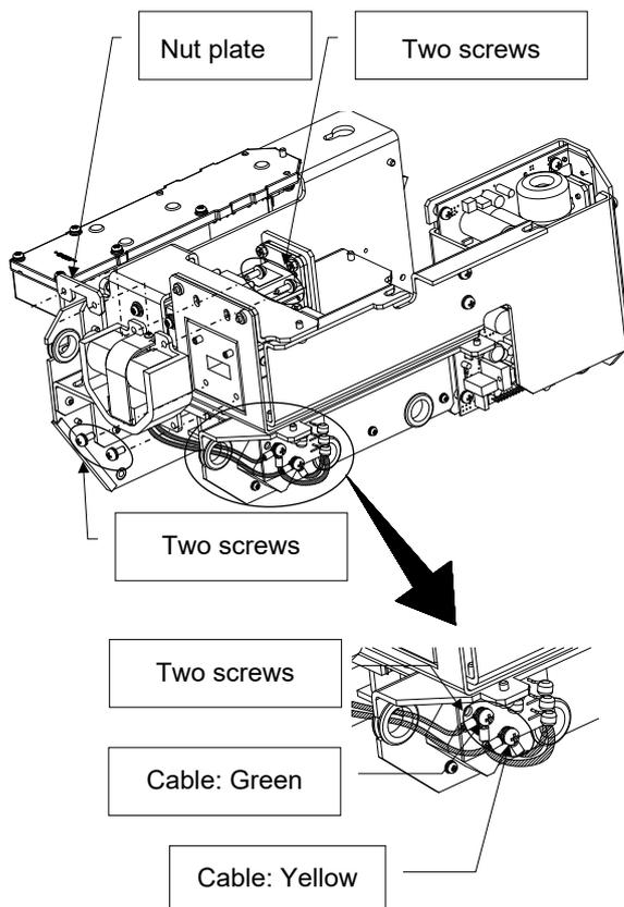
Remove two screws (M4×10), and remove the magnetron cable.
