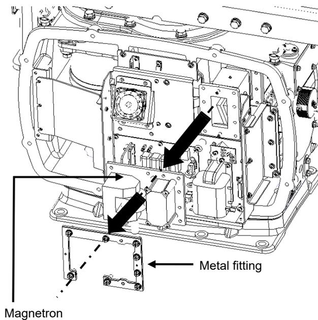
The magnetron is secured in place with a special metal fitting. The fitting uses bolts protected from falling out. Loosen all bolts and demount the fitting and bolts together.
