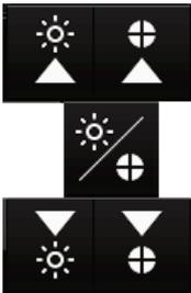
Adjust the brightness of the screen on the left side and adjust the brightness of the operation unit on the right side.
