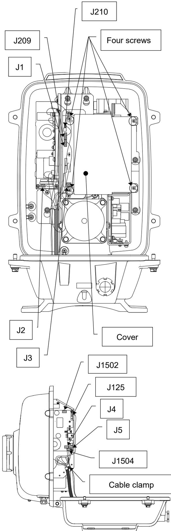
Loosen four screws (M4×12).
