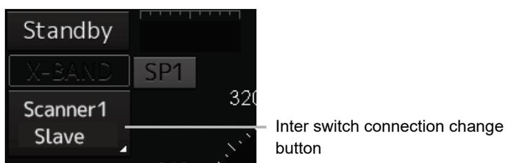
The name of the connected radar antenna is displayed in the upper part.
