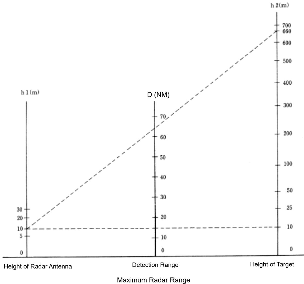
When the height of own ship's radar antenna is 10 m for instance,
