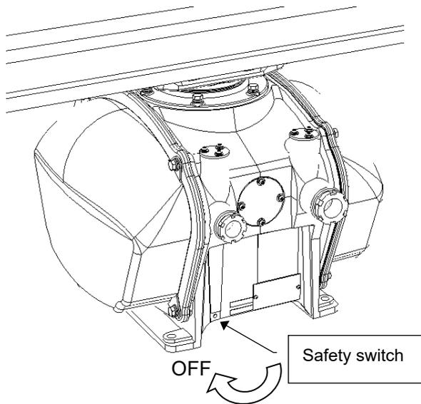
**⚠** When replacing a magnetron, ensure that the safety switch of the radar antenna is turned Off prior to commencing the replacement work.
