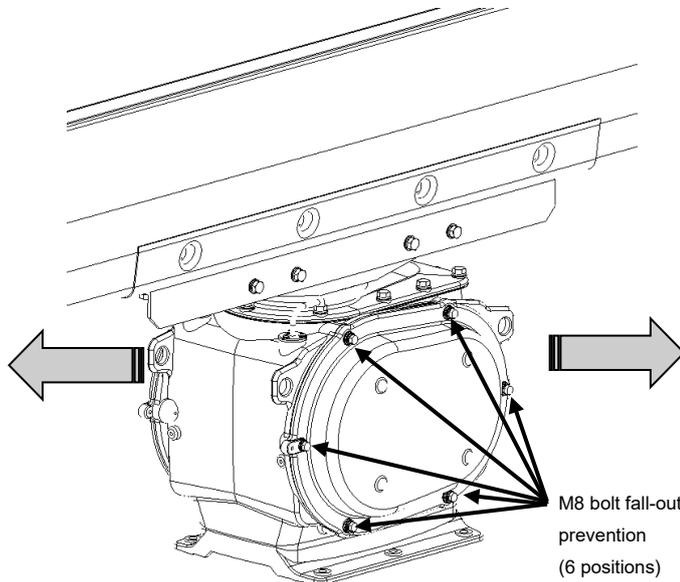
⚠ When replacing a motor, ensure that the safety switch of the radar antenna is turned Off prior to commencing the replacement work.
