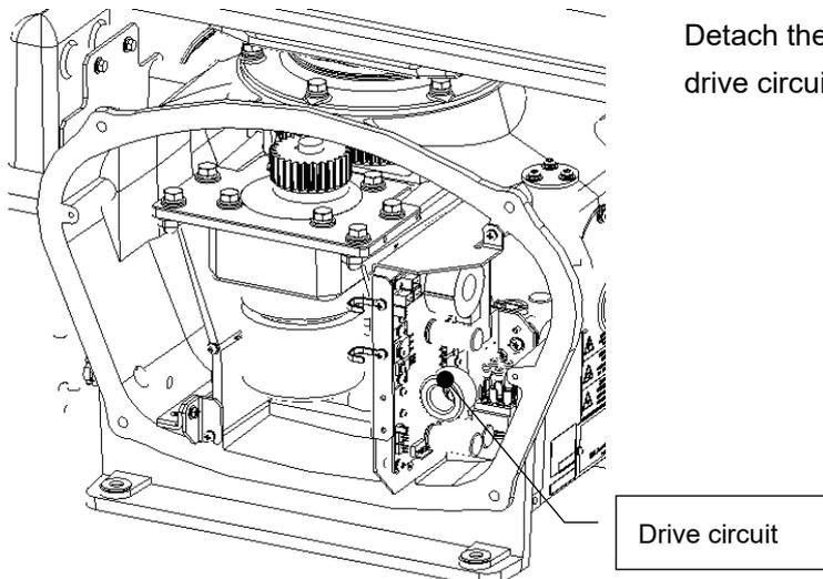
Detach the motor cable connected to the drive circuit.
