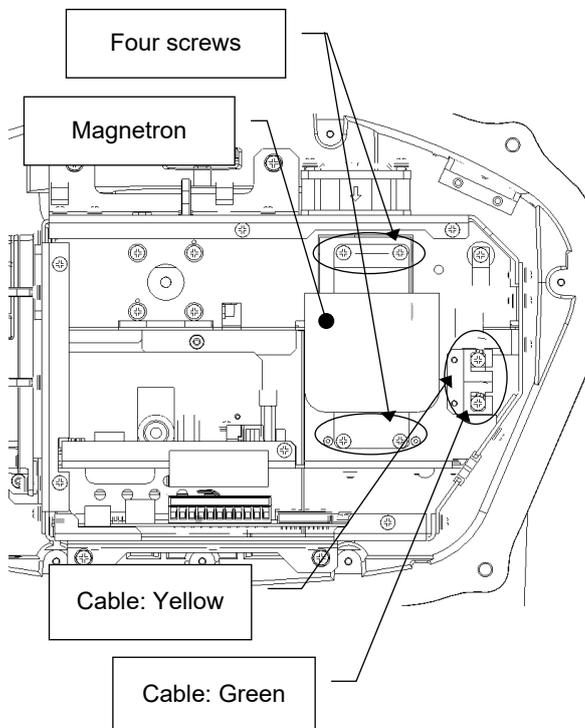
Remove two screws (M4×10), and remove the magnetron cable.
