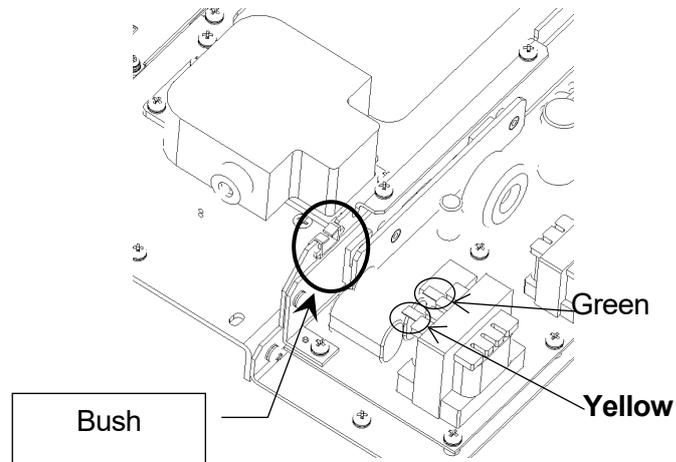
After soldering, place the cables into the bush and attach the cover.
