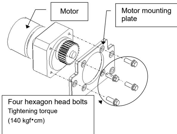
Mount the mounting plate on the motor to be replaced.
