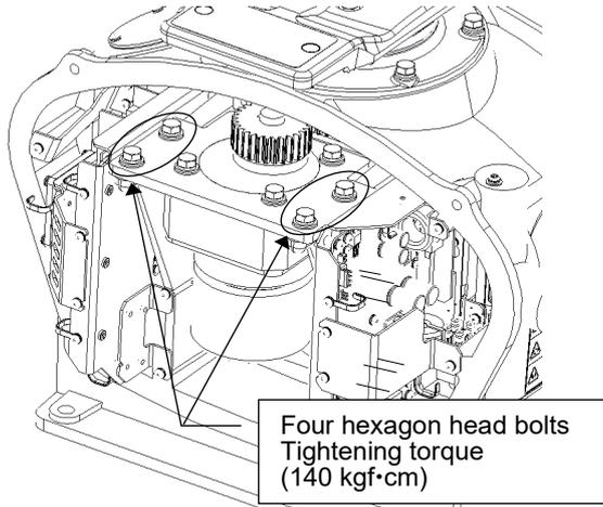
Incorporate the motor on the radar antenna.
