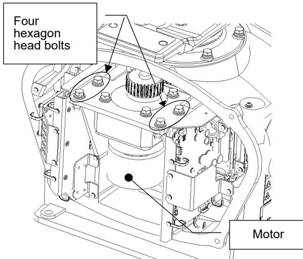
The motor is secured in place with hexagon head bolts (M8×20 SW W built-in type) at four positions.
