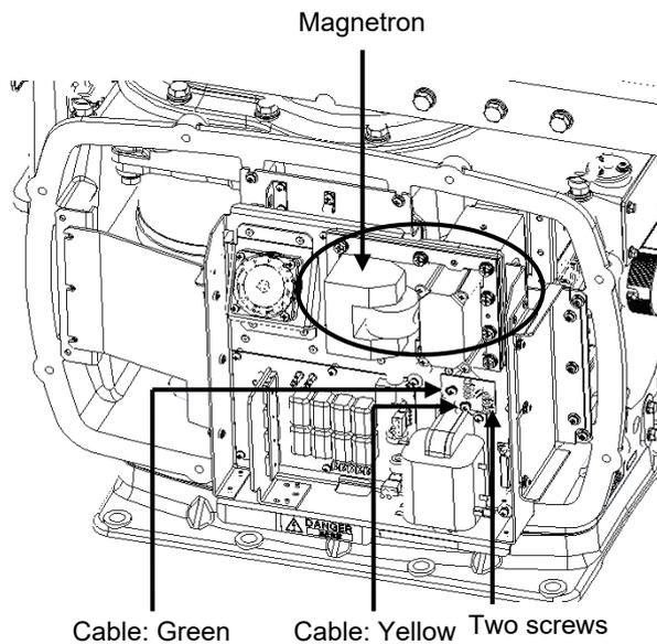
To detach the cables to which the magnetron is connected, remove the two screws (M4×12) holding the cables.
