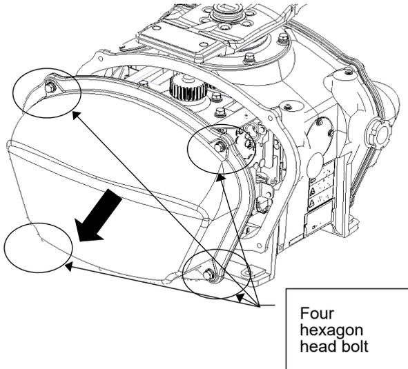
The motor is incorporated on the left side (port side) of the radar antenna. Remove the cover on the left side. The cover is secured in place with hexagon head bolts (M8, designed to be protected from falling out) at four positions.
