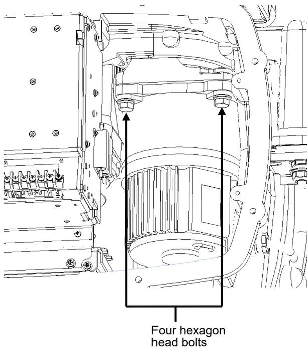
The motor is secured in place with hexagon head bolts (M10×40, SW10 and W10) at four positions.
