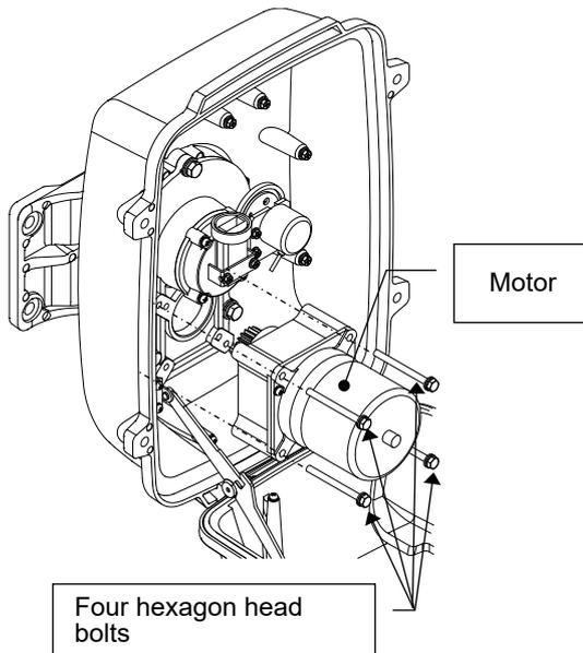
Remove four hexagon head bolts (M6×70), and remove the motor.
