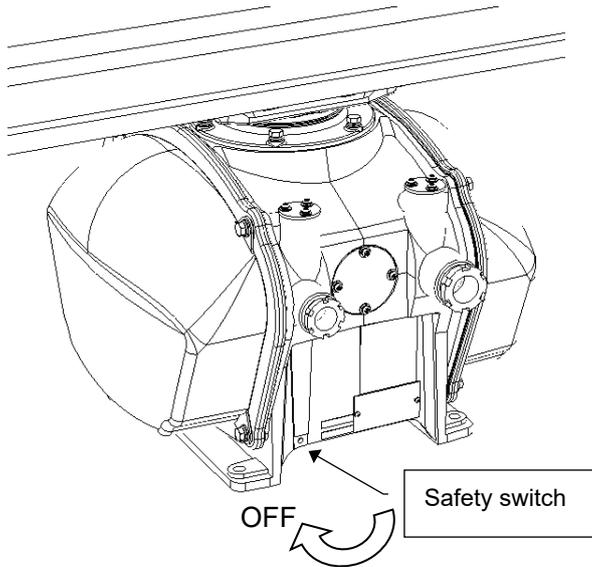
**⚠** When replacing a motor, ensure that the safety switch of the radar antenna is turned Off prior to commencing the replacement work.
