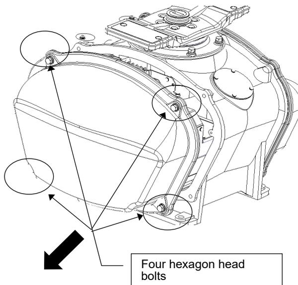
The magnetron is incorporated on the right side (starboard side) of the radar antenna. Remove the cover on the right side.
