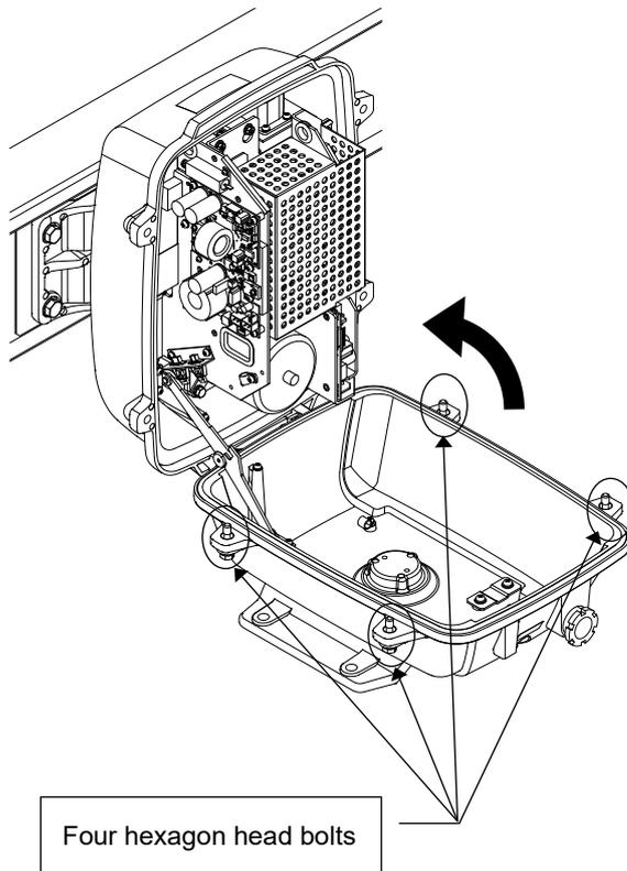
The upper cover is secured in place with hexagon head bolts (M8, designed to be protected from falling out) at four positions.
