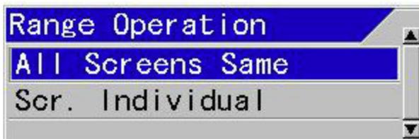
7. When [MENU] key
