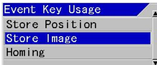
7. When [MENU] key
