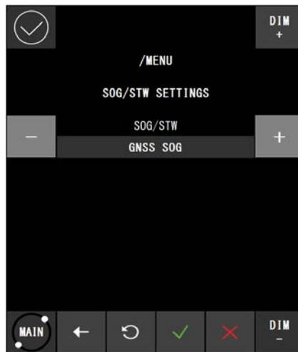
GNSS SOG: Speed over the ground by the satellite log (initial value)
