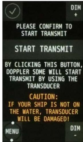
When the [START TRANSMIT] button is touched, the normal screen is displayed. Transmission starts.
