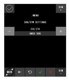
GNSS SOG: Display the vessel speed over ground from the GPS compass sensor.
