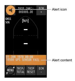
Press the alert content, the buzzer sound stops
