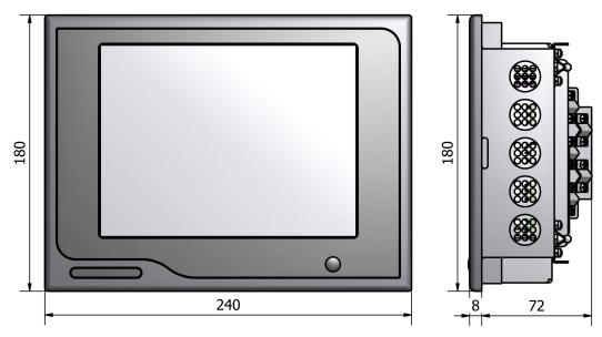
Weight: 2.4kg NWZ-840SDR (Unit: mm)
