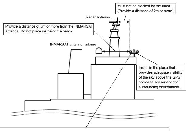
Provide a distance of 2m or more from the radar antenna.
