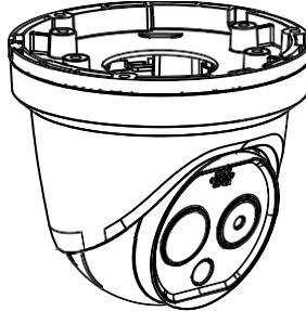
Figure 2-2 Type II Thermal Turret Camera Overview
