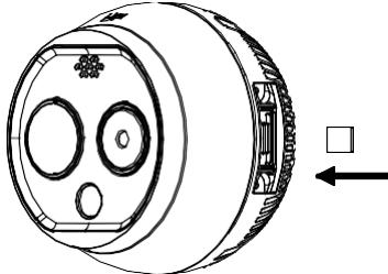
Figure 3-2 SD Card Slot
