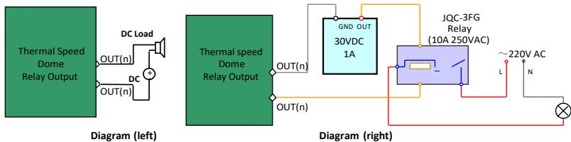
Figure 2-4 Alarm Out Connections
